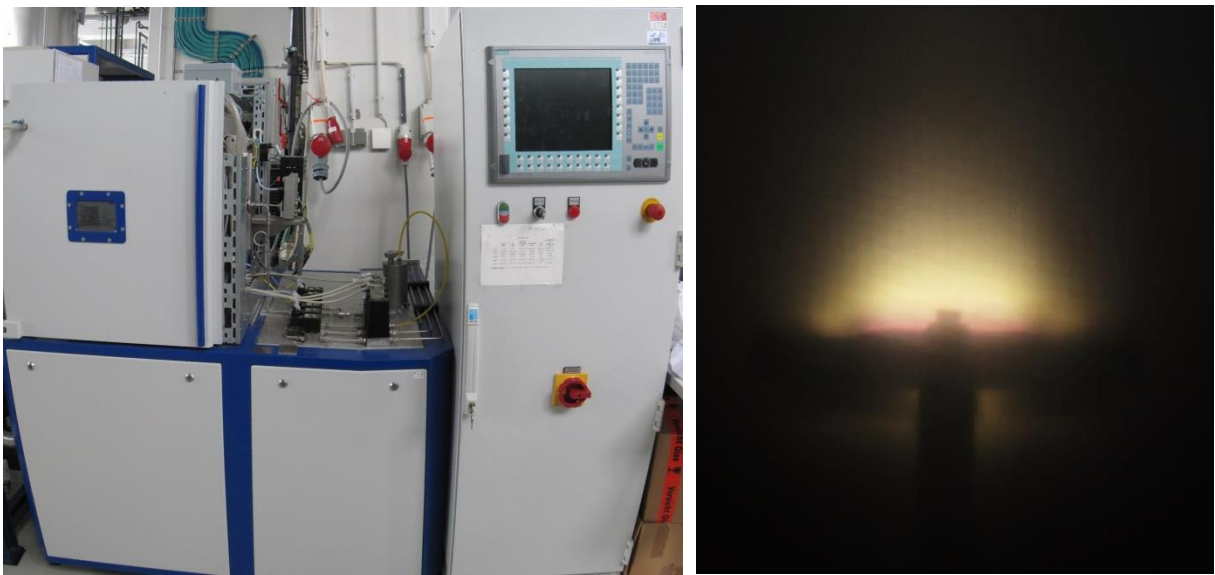
Figure 2.3: Plasma device and the image of the O 2 etching process.
