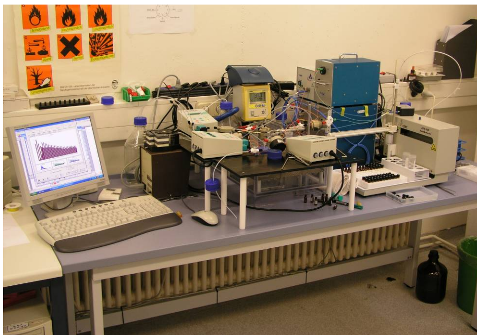
Figure 4.2. Photograph of the automated setup. The SIA devices are placed on the right side, the water bath in the middle, and the controlling computer on the left side.
