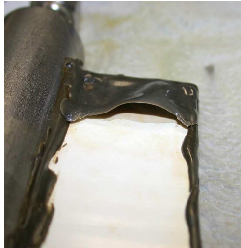
Fig. 6.5: The epoxy adhesive lost binding when autoclaved with surfactant.
