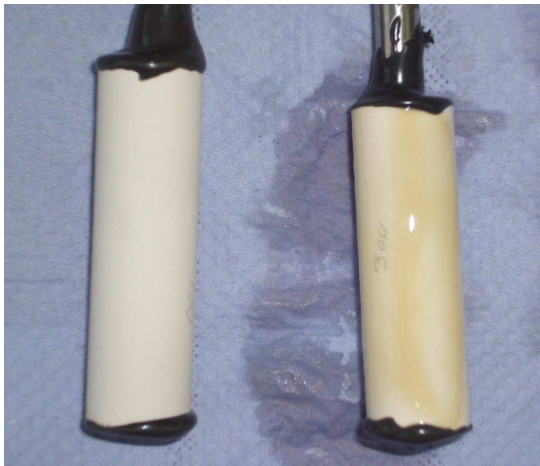
Fig. 5.5: Visual comparison of membrane for biofouling: membrane after one hour filtration (right), unused membrane (left).
