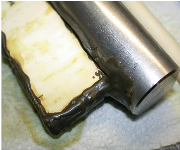
Fig. 5.2: Irreversible biofouling, no significant cell layer could be seen on the membrane surface and the surface could be regenerated by simple washing under water.
