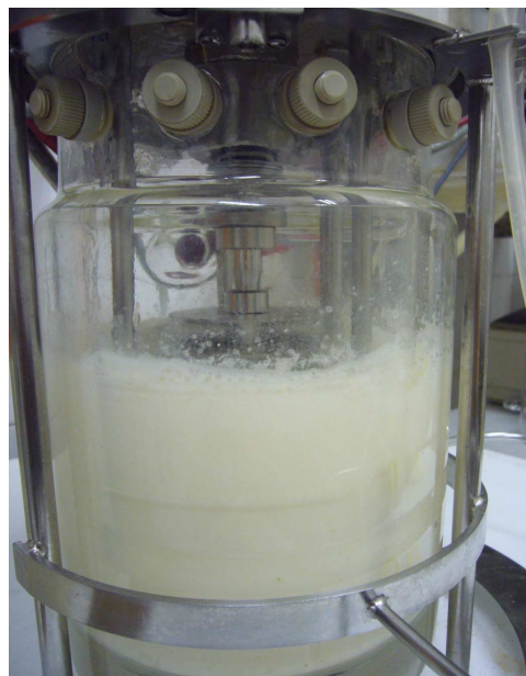
Fig. 6.12: Effect of emulsified feeding; the foam production was significantly reduced and hence the loss of culture volume was completely controlled.
