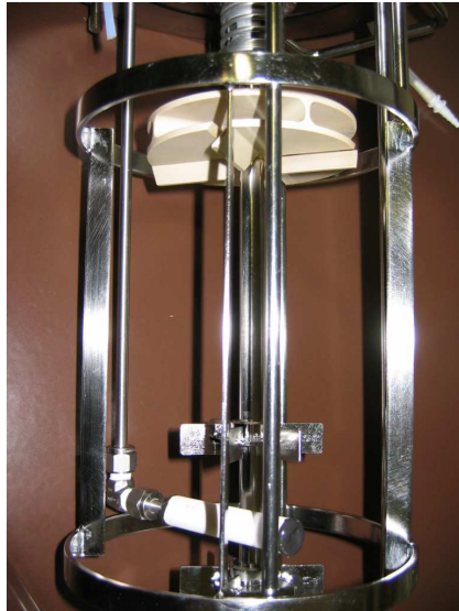
Fig. 6.2: Cylindrical ceramic membrane fitted in the bioreactor for emulsified feeding of oil.
