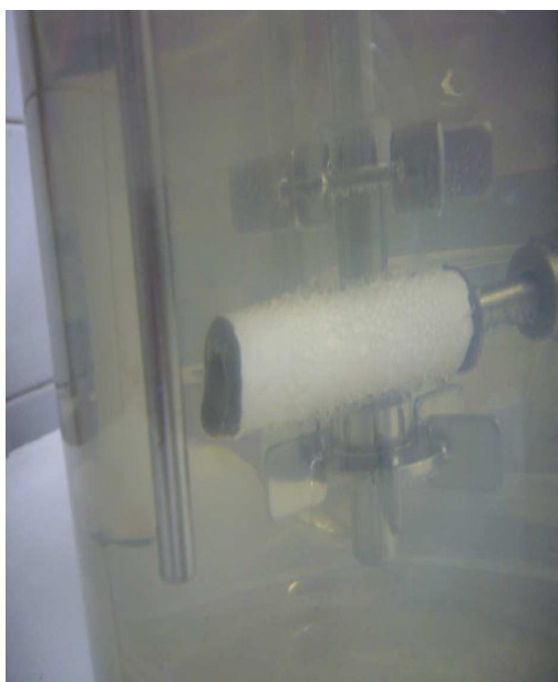
Fig. 6.11: Emulsification via submerged membrane, fine oil droplets could be seen here coming out at the membrane surface.
