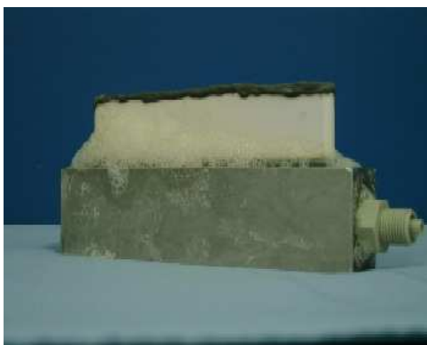
Fig. 4.6: Optical examination of a membrane after a long-term test (filtration time 30 minutes; periodic break in operation 3 minutes).
