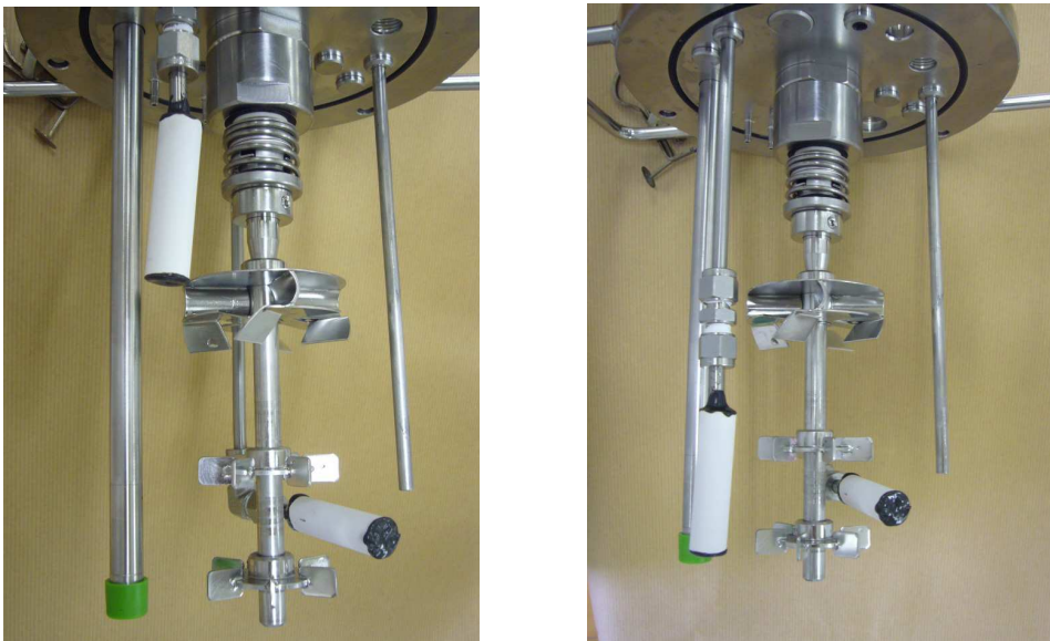
Fig. 5.13: Adjustable arrangement of integrated membranes, monochannel ceramic membranes integrated with in the bench scale bioreactor for product recovery. The first membrane was placed between the impellers to provide maximum turbulence over the membrane surface. The second membrane was placed in the head space above the antifoam disk (left) and was immersed into the culture (right) when the cells were in stationary phase.
