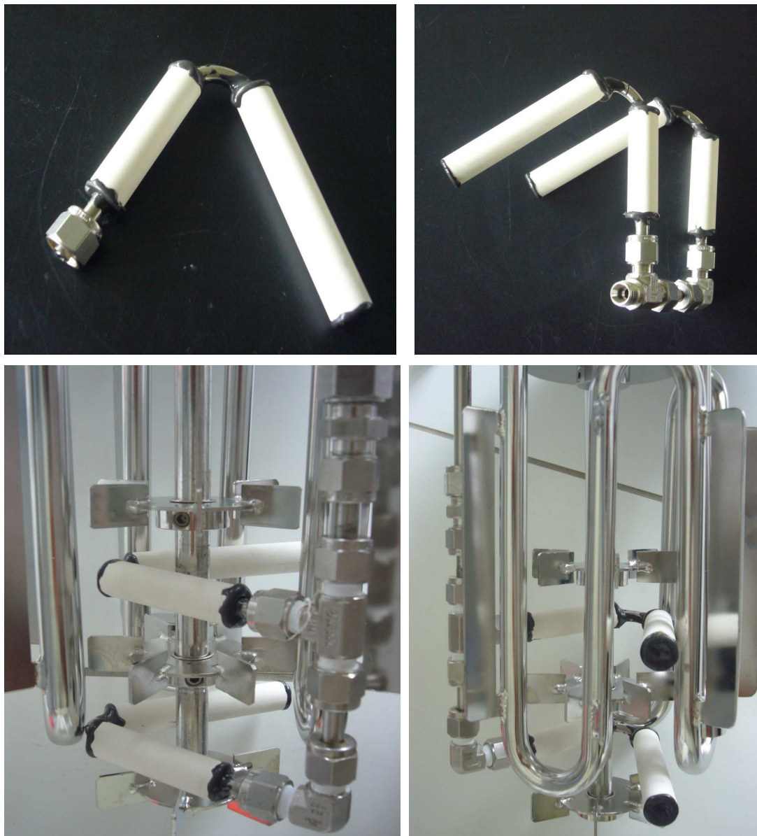
Fig. 4.10: The \Lambda module: the available filtration area was approx. 105 \text{ cm}^2 . The membranes could be fitted safely inside the stainless steel cage of the bioreactor. Cylindrical membrane attached via a steel tube (above) and the whole module fitted into the bioreactor (below).
