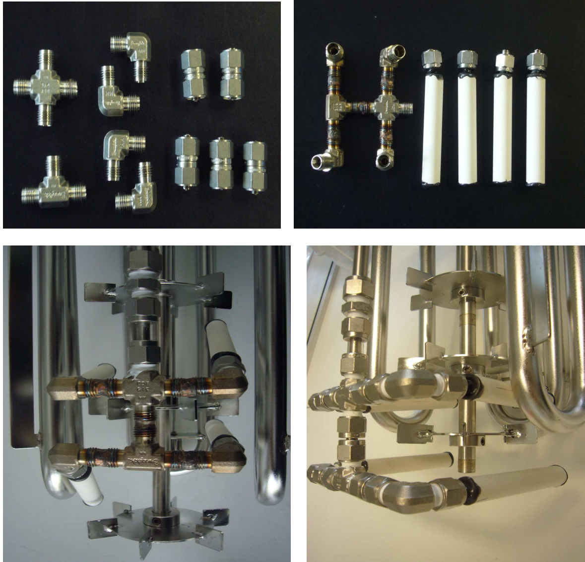
Fig. 4.12: The \Pi module: the available filtration area was approx. 140 cm 2 . The membranes could be fitted safely inside the stainless steel cage of the bioreactor and the integrated membranes could be rotated to adjust to the available space. Stainless steel fitting and the resulting module and membranes (above) and the whole module fitted into the bioreactor (below).
