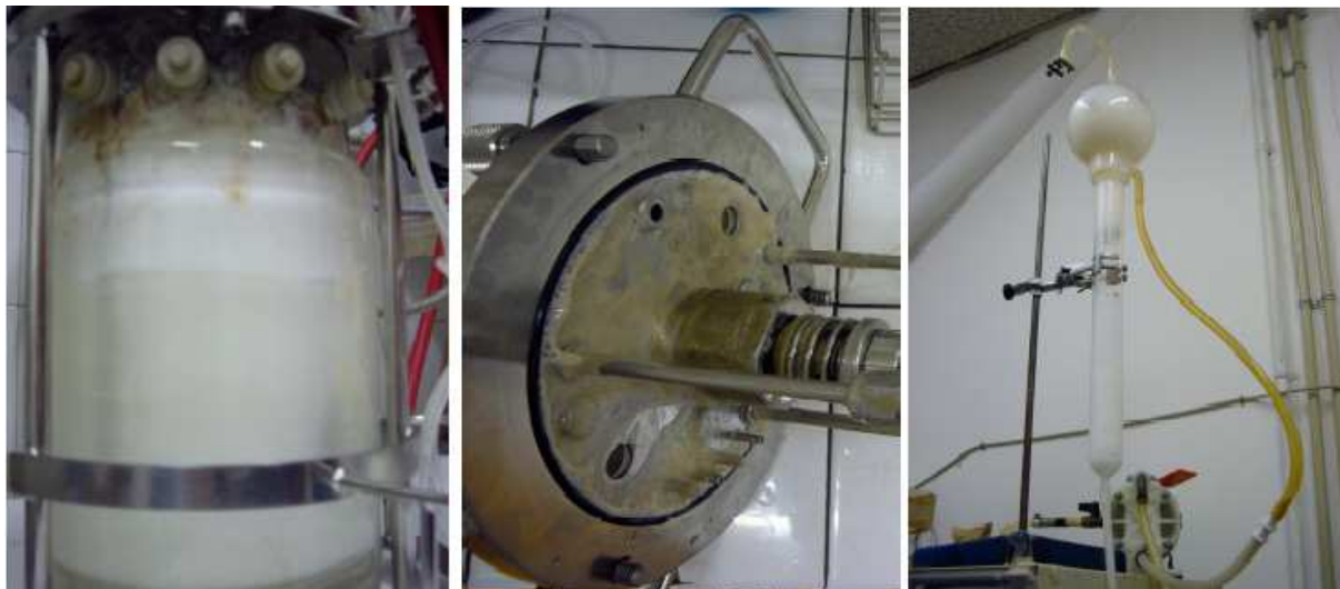
Fig. 6.8: The foaming problem during the batch process for PHA production with P. aeruginosa 42A2: the bioreactor is full with foam even when employing only 50% working volume (left), most of the cells reach the top cover of the reactor with the foam and stick there forming biofilms (center), the overhead column connected to the exit gas port for collection and breaking of foam is completely full with foam and a lot of foam flows out and could not be recycled back to the bioreactor (right).
