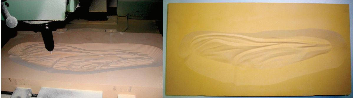
Figure 6. Milling of the cavity and the finished form
