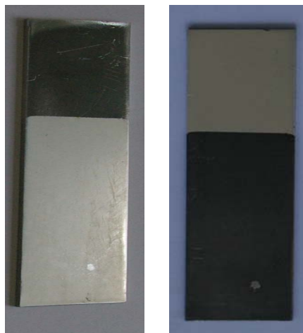
Fig. 6-39: Selective Ni-Al_2O_3 coating derived from an aqueous nickel nitrate-Alu C suspension (suspension A) before and after reducing in H_2 atmosphere at 450 °C
