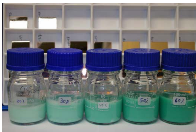
Fig. 6- 36: Prepared aqueous suspensions with different nickel contents for deposition of cermet layers
