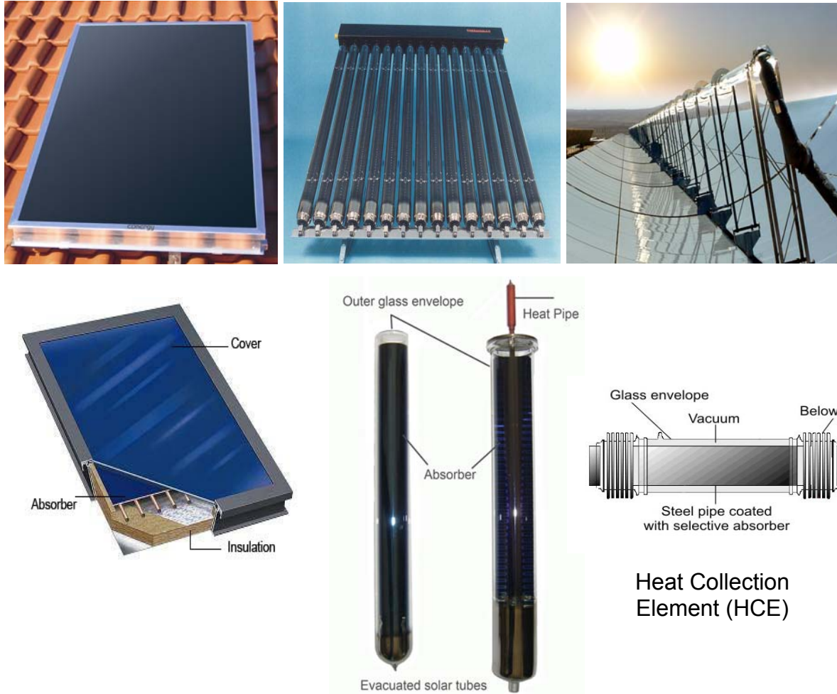
Fig. 3-1: Different kinds of solar thermal collectors (upper row) and their components (lower row). From left to right: Flat-plate collector, evacuated absorber tube and parabolic concentrated collector
