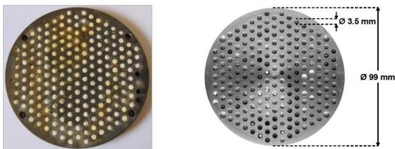
Figure 7.4 Image of a stainless-steel library plate with catalyst samples
