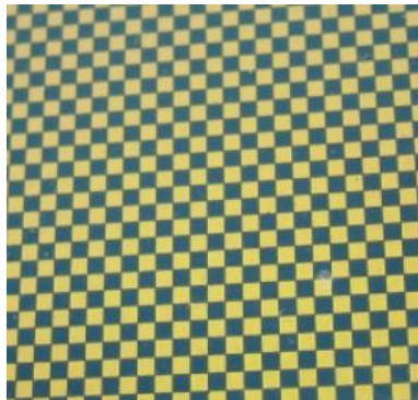
Fig. 6-8 Chess board created by multiline (two adjacent) addressing in the DDS of Ch-LCD
