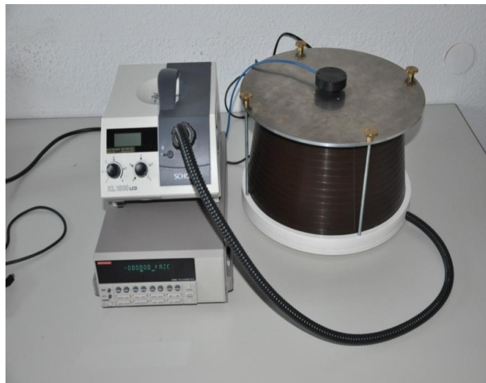
Fig. 8-9 Reflectance measurement set
