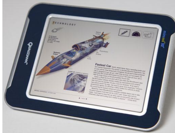
Fig. 1-14 IMOD display by Qualcomm (5.7" XGA format (1024 x 768 pixels))
