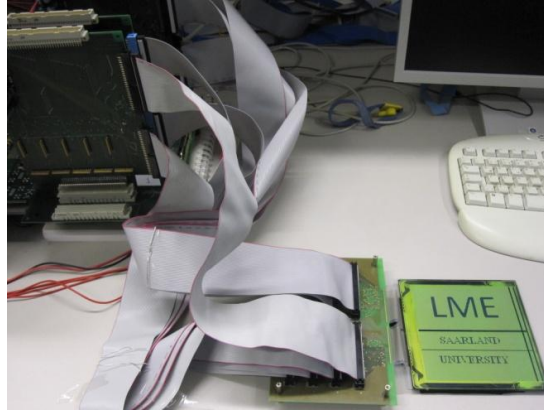
Fig. 3-20 160 rows cholesteric LCD is driven by the proposed DDS
