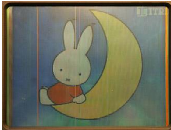
Fig. 1-9 10.4 inch QVGA single layer color Ch-LCD by ITRI
