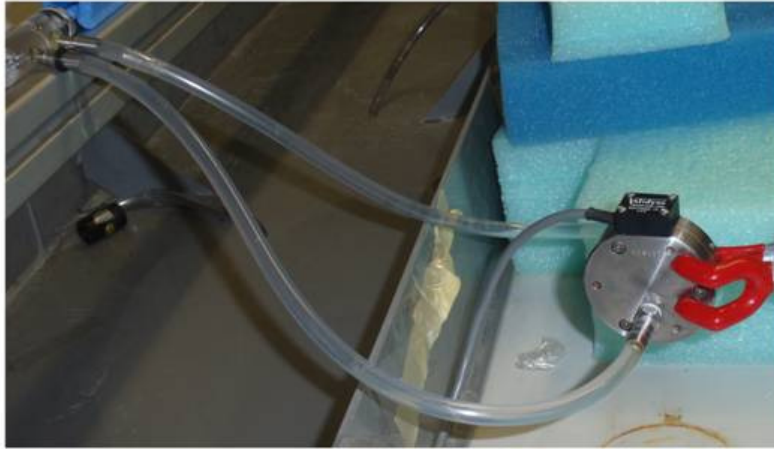
Figure 4.6: A Validyne pressure sensor connected to a pipe setup
