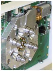
(a) Active docking unit on a lateral side of Kabot
