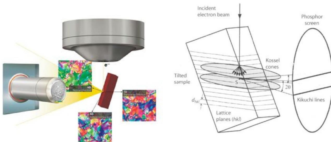
Figure 3.2: Schematic EBSD measurement configuration (left 5 ) and formation of the Kikuchi patterns (right) [67].
