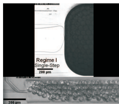
SI 1 Overview of the different breakup regimes by example movies taken in the two geometries used. Top row: Geometry A ( w/b = 30 ) Bottom row: Geometry B. Movies recorded at different framerates, cf. timestamp.
