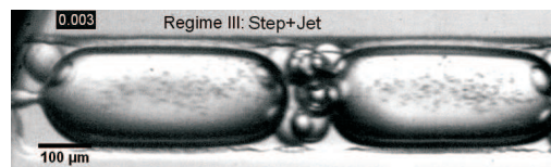
SI 4 Video exemplifying the simultaneous concentration and encapsulation of PMMA particles ( \phi 4 \mu\text{m} ) by coexistence of step- and jet-instabilities on a single filament in Geometry B.
