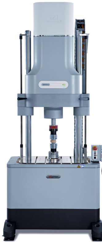
Abbildung 5.9: Instron ElectroPuls E10000 Linear-Torsion.
