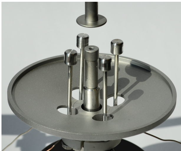
Figure 3.2 – Electrode system of the mobile electrostatic levitator.
