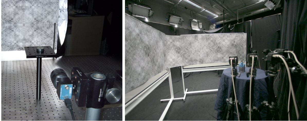
Fig. 8.6. The single camera setup (left) and the camera array (right) that we use for acquisition.
