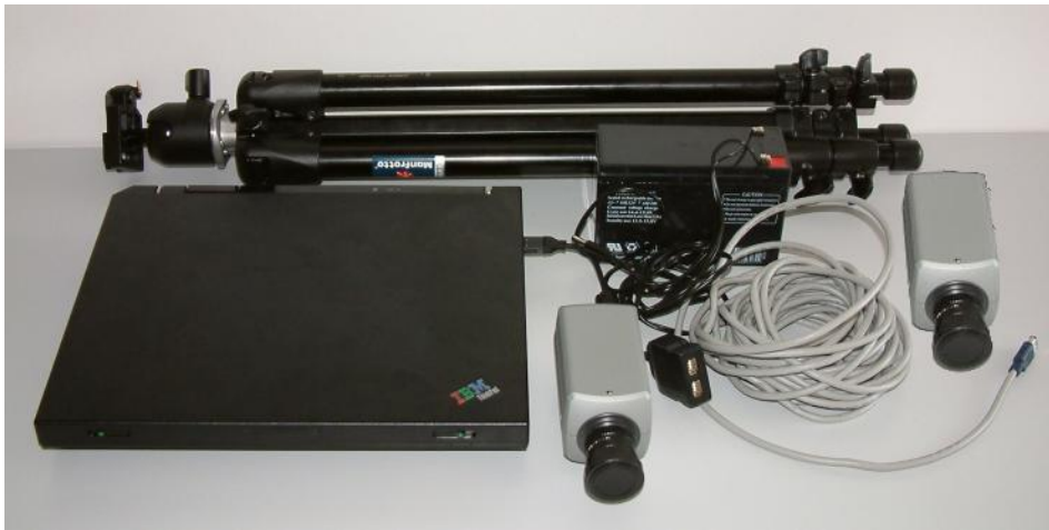
Fig. 4.2. One module of the mobile recording system [4]: it consists of two cameras, a laptop for controlling the acquisition, a rechargeable battery to power the cameras, a tripod and some wires.
