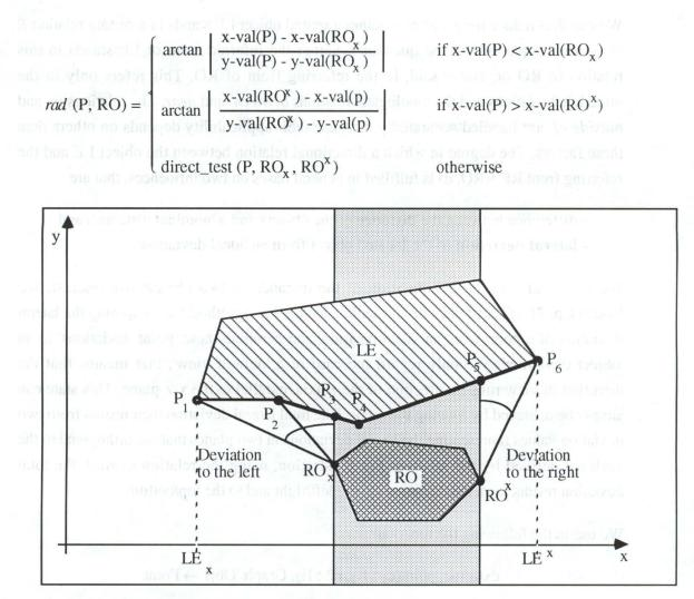
Fig.5 : Computation of the average lateral deviation
