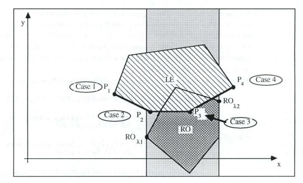
Fig.7 : Computation of the lateral deviation
