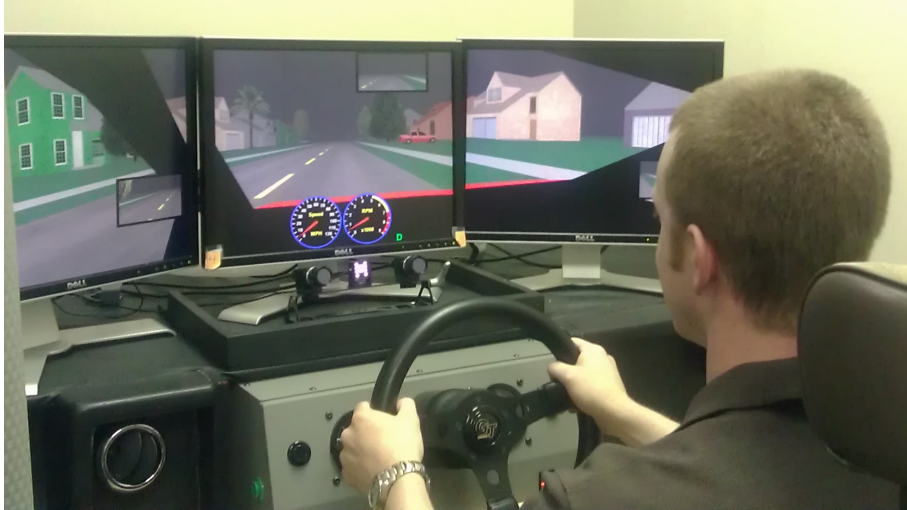
Figure 2.1: STISIM (M500) setup (source: [6])
