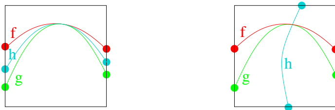
Figure 4.3: The Jacobi curve h either cuts tangentially or transversally through a non-singular tangential intersection point of f and g .
