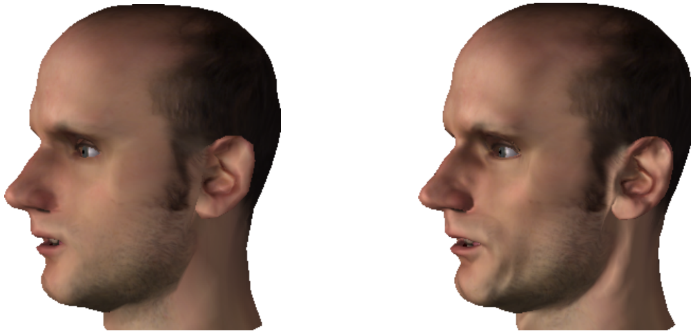
Figure 9.3: Head model rendered as standard triangle mesh (left, 2030 triangles) and displaced subdivision surface on that mesh (right, 2 refinement levels)
