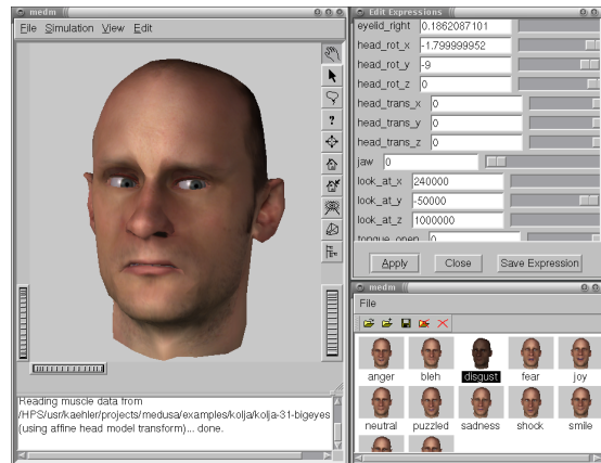
Figure 5.5: Expression Editor. Left: current expression shown in the running simulation; top right: adjustable muscle parameters; bottom right: expression palette.
