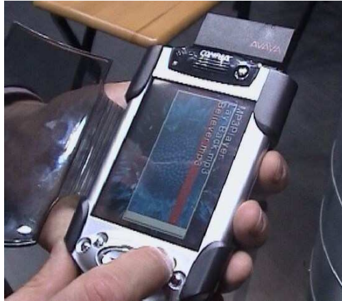
Figure 15.4: The iPAQ 3870 using an expansion jacket holding a PCMCIA card for WLAN access [NMMa].
