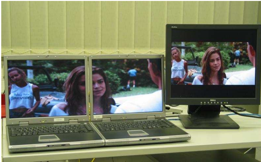
Figure 13.2: A video wall using two laptop computers as clients and a third system connected to an LCD as server. The clients only render cropped sections of the video stream; the server shows complete video frames. Audio output is also performed on the server. NMM provides inter-stream synchronization for all connected systems.
