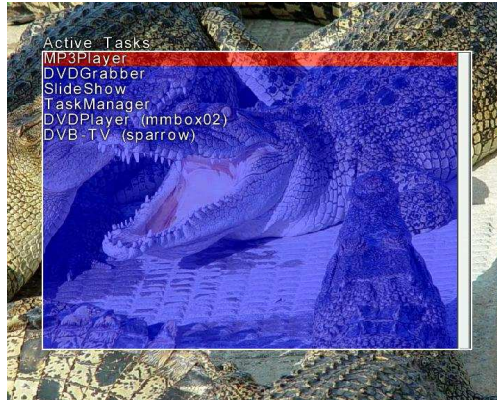
Figure 15.9: The user interface of the tasklist state of the Multimedia-Box. States running locally in the background can be reactivated or terminated. States running on distributed systems are labelled with the name of the corresponding host and can be joined by using the facilities of the session sharing service.
