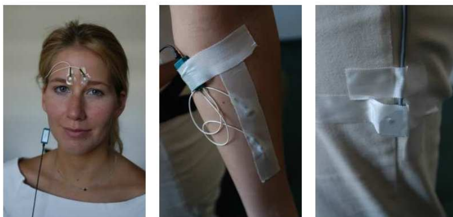
Figure 9.2: The three bio sensors (a) Electrooculogram (EOG) , (b) Electromyogram (EMG) and (c) Acceleration (ACC) according to [Brandherm and Schmitz, 2004]
