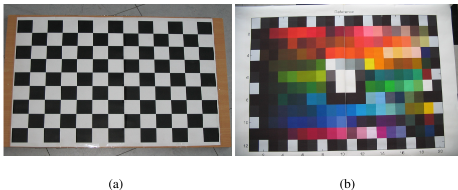
Figure 4.3: (a) Small checkerboard used for intrinsic parameter estimation. (b) Color pattern used for multi-view color adjustment.
