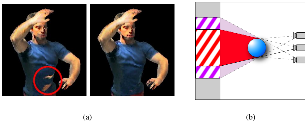
Figure 8.14: (a) Small differences between object silhouette and model outline cause erroneous texture projections. (b) By projecting each video camera's image onto the model also from slightly displaced camera positions, regions of dubious visibility are determined (purple) which are then not textured by the camera.
