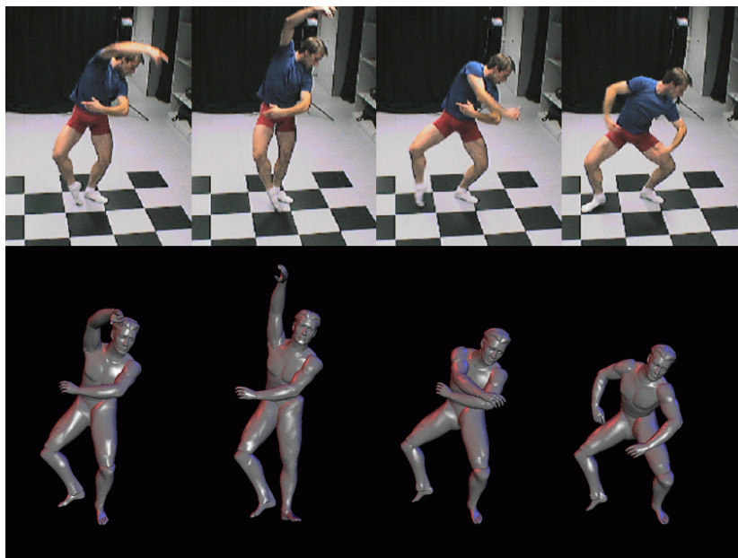
Figure 8.7: From eight image silhouettes per time step, model-based analysis automatically captures the complex motion of a ballet dance performance.
