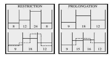
**Fig. 4.2**: One-dimensional example for an area based restriction operator  $R^{\mathbf{h}\to\mathbf{H}}$  and an area based prolongation operator  $P^{\mathbf{H}\to\mathbf{h}}$  with  $\frac{\mathbf{h}}{\mathbf{H}} = \frac{3}{4}$ . Numbers denote grey values. Grey values are weighted proportional to their area, e.g.  $\frac{3}{4}8 + \frac{1}{4}12 = 9$ .
