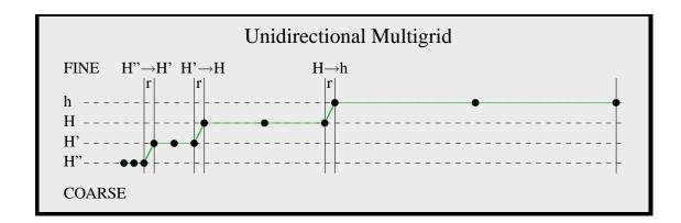
**Fig. 4.1**: Schematic drawing of a unidirectional multigrid strategy. Starting from a very coarse variant of the original equation system, the solution is refined step by step. The corresponding refinements steps are marked with 'r'. At each resolution level several iterations with the basic solver are performed. This is indicated by large black dots.
