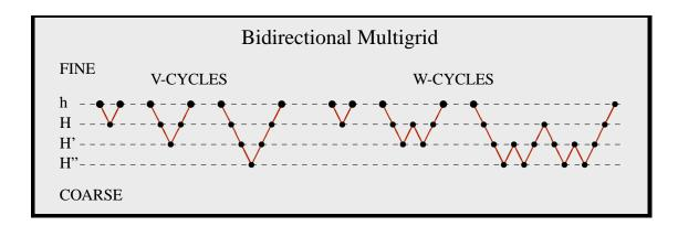
**Fig. 4.7**: Schematic drawing of bidirectional strategies (V– and W-cycles) for two, three and four levels. Iterations with the basic solver on the original problem are marked with large black dots, while iterations on residual problems are symbolised by small black dots.
