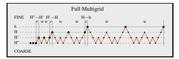
**Fig. 4.9**: Schematic drawing of a full multigrid strategy, Starting from a very coarse variant of the original equation system, the solution is refined step by step. The corresponding refinements steps are marked with 'r'. At each resolution level two W-cycles are used as solver. Each of these cycles is marked with 'w'. Iterations with the basic solver on the original problem are represented with large black dots, while iterations on residual problems are symbolised by small black dots.
