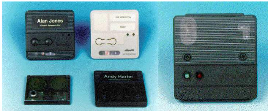
Figure 3.6: left: Four generations of active badges, right: the networked sensor (source: http://www.uk.research.att.com/ab.html )
