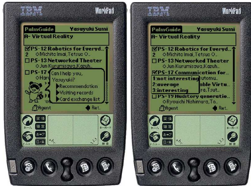
Figure 3.28: Virtual character overlay and user query on a PDA in PalmGuide (source: Sumi & Mase, 2001a)
