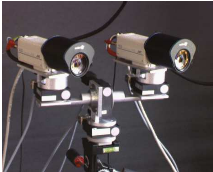
Figure 2.6: A binocular camera head, equipped with two RGB cameras, to determine and interpret human pointing gestures (source: Rae & Ritter, visited 2005)
