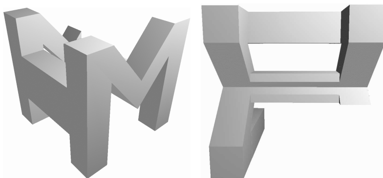
Figure 10.2: Two views on a visual hull example created from three two-dimensional silhouettes showing the capital letters M, P, and I.
