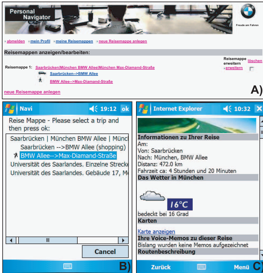
Figure 2.9: Downloading a travel itinerary onto the PDA: A) the desktop interface and B), C) the navigation routes and route information as they appear on the PDA. Note also the ‘walking’ and ‘car’ icons which denote whether a particular route is for pedestrians or for automobiles.
