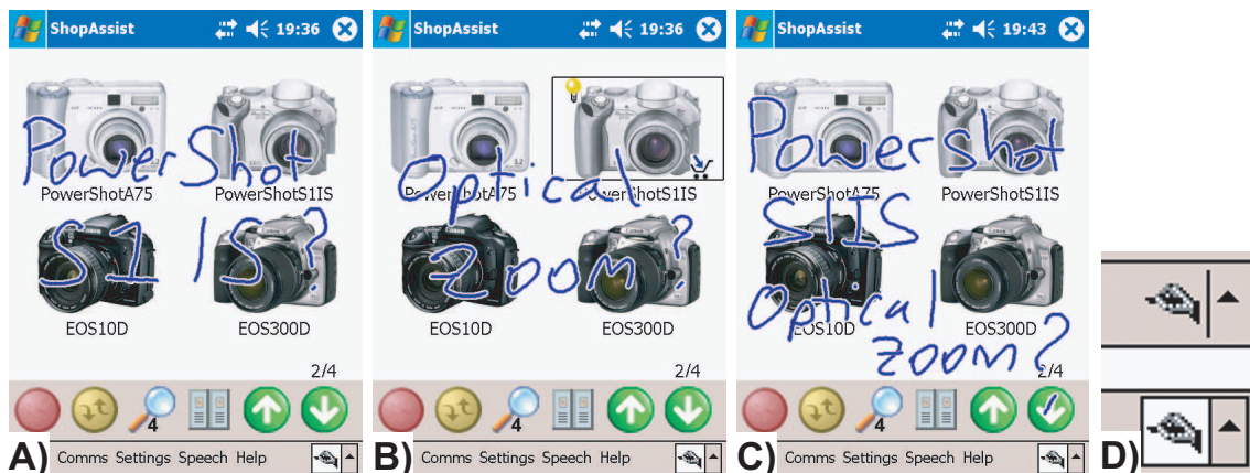
Figure 4.5: The use of handwriting-only input in the MSA for selecting A) an object, B) a feature, and C) both a feature and an object. D) shows the graphical button used to activate the handwriting recognizer in its deactivated (top) and activated (bottom) state.
