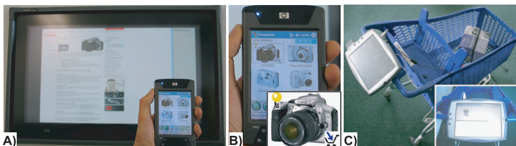
Figure 2.19: MSA ties to the instrumented environment, showing A) a public display, B) the on-device shopping basket to which Mr. S added the product (see inset), and C) an RFID-instrumented shopping trolley that can be combined with the MSA (Schneider, 2004).
