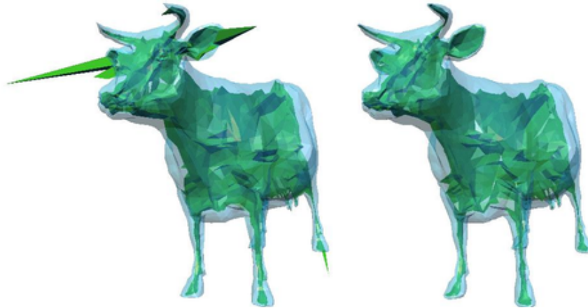
Figure 6.6: Left: a cow mesh and its inner skeletal mesh, notice that the skeletal mesh intersects the cow mesh. Right: the cow mesh improved by several iterations of the bilaplacian tangent flow and its skeletal mesh improved original cow mesh via 100 bilaplacian tangent flow provides a good skeletal mesh.
