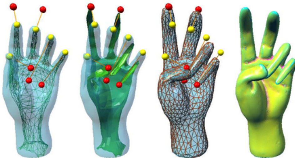
Figure 6.16: Skeleton-based deformations enriched by DSS: the hand model has 38K triangles while its skeletal mesh consists of 2K triangles only.
