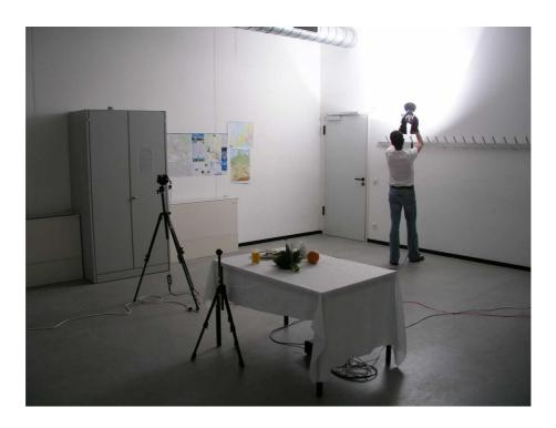
Figure 7.4: Measurement setup for the still camera: an Olympus C5050Z digital camera records objects on a table which are indirectly lit by a hand-held spotlight pointed at the white walls, ceiling and floor. The reference object, a black snooker ball, is mounted on the small tripod next to the table.
