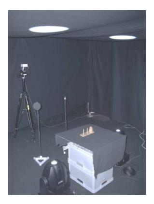
Figure 4.1: Photograph of our measurement setup. Spot light projectors on the floor shine on a tent made from black cloth, and the bounce light illuminates the scene, which is arranged on top of the boxes. A tripod-mounted camera records the scene, and is protected against lens flares by occluders. In order to show the inside of the tent, we have added additional illumination (lamps outside the picture) which is not present during the acquisition.
