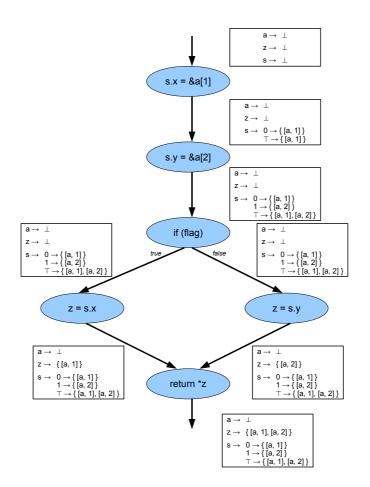
Figure 5: Control flow graph for code from figure 4 with analysis results
