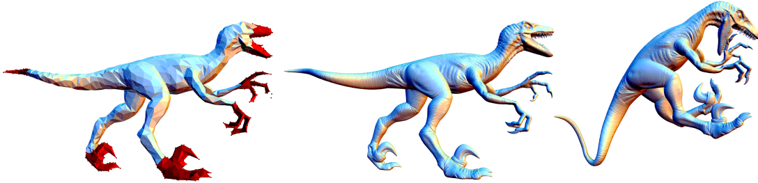
Figure 8.1: Example of a deformation of a raptor created with our method. From left to right: Reduced tetrahedral model with handles in red, original high resolution input model, deformed input model.
