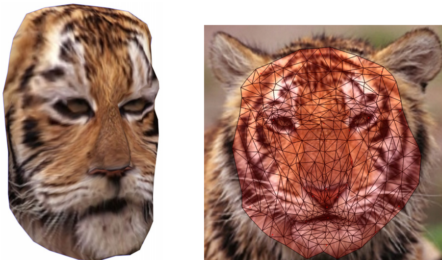
Figure 4.6: Using the vector fields to calculate a planar parameterization of the mesh. The picture shows the texture mapping of a tiger image onto the face model (left) and the corresponding parameterization domain (right).
