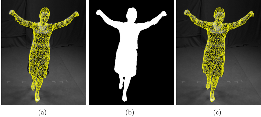
Figure 6.4: Model refinement using 2D image constraints : (a) Input model overlaid on camera image. (b) Segmented silhouette image. (c) Refined model overlaid on camera image. Note the increased accuracy especially on the skirt.
