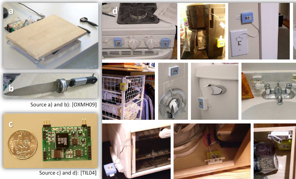
Figure 9.9: Additional sensors in the kitchen: Instrumented knife (a), cutting board with load sensors (b), and cheap state change sensors (c) at various places in the home (d).
