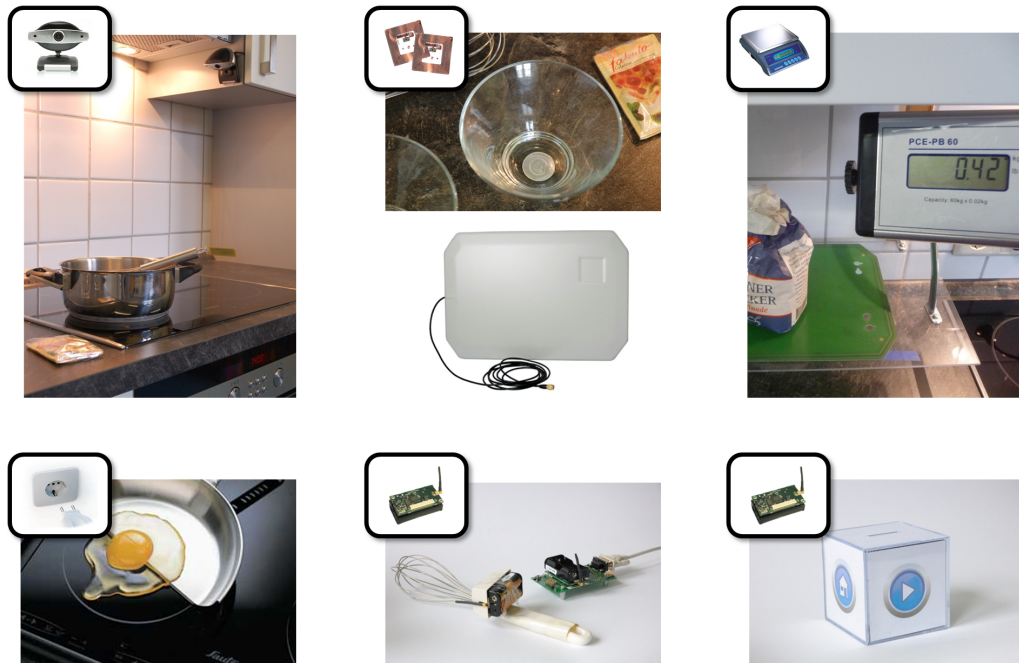
Figure 9.2: Sensors of the Smart Kitchen : Cameras (top left), RFID reader (top center), digital scale (top right), networked appliances (bottom left), instrumented tools (bottom center), and control cube interface (bottom right).
