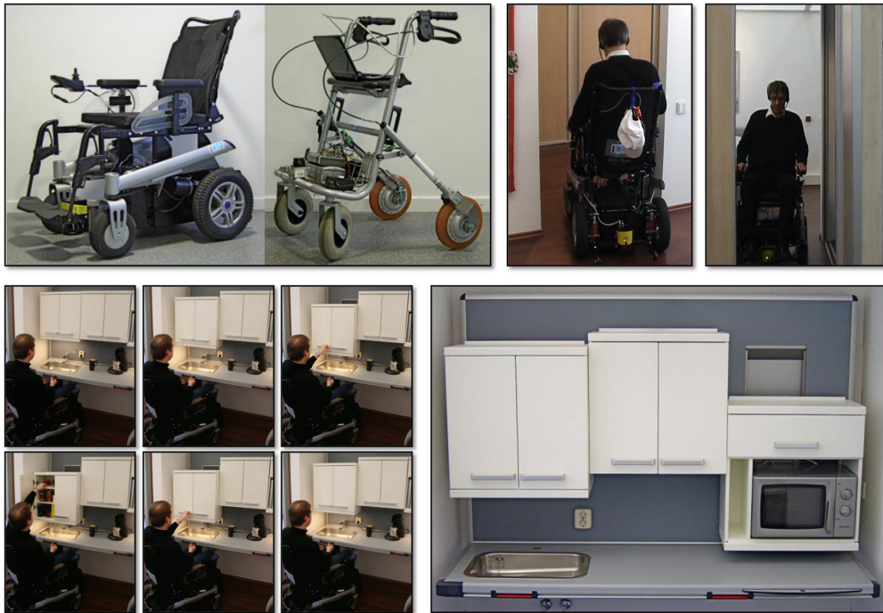
Figure 5.2: The Bremen Ambient Assisted Living Lab supports elderly and impaired people in their everyday living, e.g. by autonomous navigation of a smart wheelchair and walker (top), or by proactively adjusting the height of kitchen shelves to the user’s needs (bottom). Source: [Ger09a].
