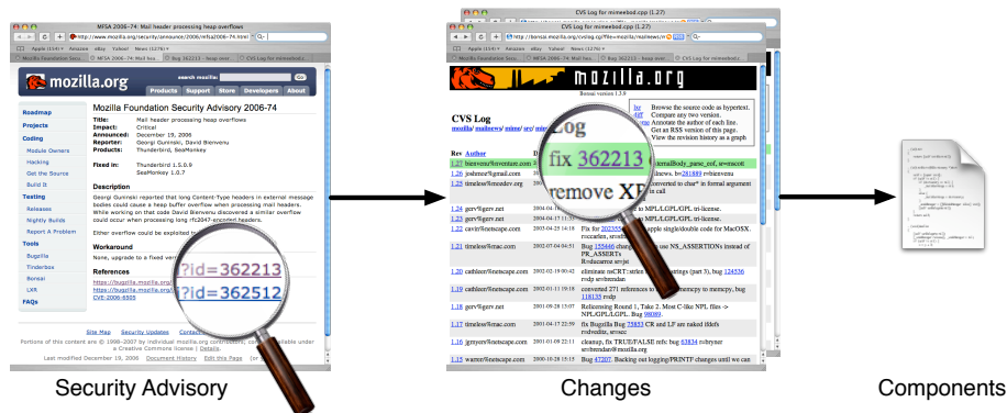
Figure 6.3: Mapping Mozilla vulnerabilities to changes. We extract bug identifiers from security advisories, search for the fix in the version archive, and from the corrected files, we infer the component(s) affected by the vulnerability.
