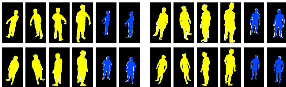
FIGURE 6.12: Four 3D scans of different subjects are projected into virtual cameras. Shape estimation is performed and the result is overlaid into the input images (yellow). The two additional images show that the estimation fits well also in views that were not used in the optimisation (blue).
