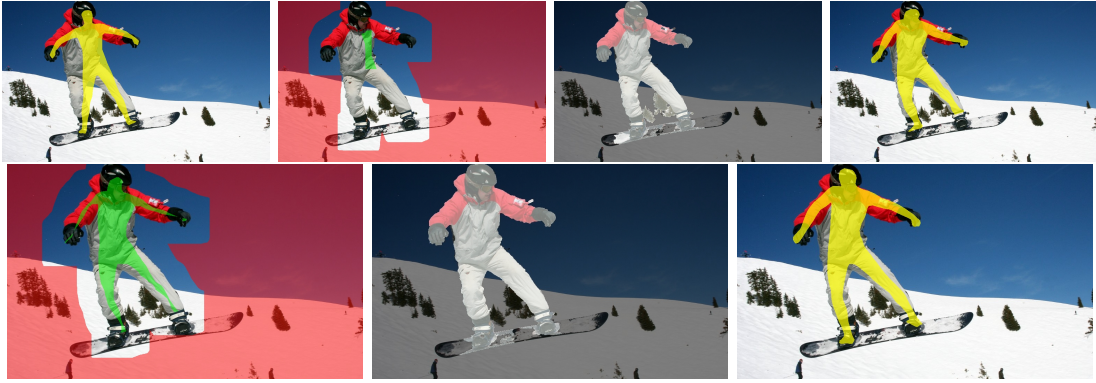
FIGURE 6.21: Automatic foreground segmentation. Top row (from left to right): Initial estimate using four markers, input to GrabCut, output of GrabCut, and estimation result. Bottom row : Second iteration of the approach. GrabCut input, GrabCut output, and result are shown.
