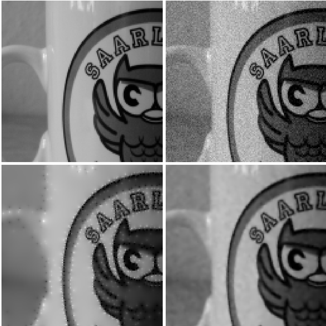
Figure 1.2: Higher order nonlinear diffusion with g(s^2) = 1/(1 + s^2/\lambda^2) . Top left : Original image, 256 \times 256 pixels. Top right : With additive Gaussian noise, standard deviation \sigma = 10 . Bottom left : Method by You and Kaveh [213] without postprocessing, \lambda = 2.5 , t = 100 . Bottom right : Method by Lysaker et al. [122] \lambda = 0.01 , t = 6 .
