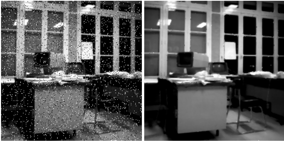
Figure 5.5: Denoising experiment in 2-D with impulse noise. Left: Test image ( 256 \times 256 pixels) with salt-and-pepper noise. Right: Denoised version of the image.
