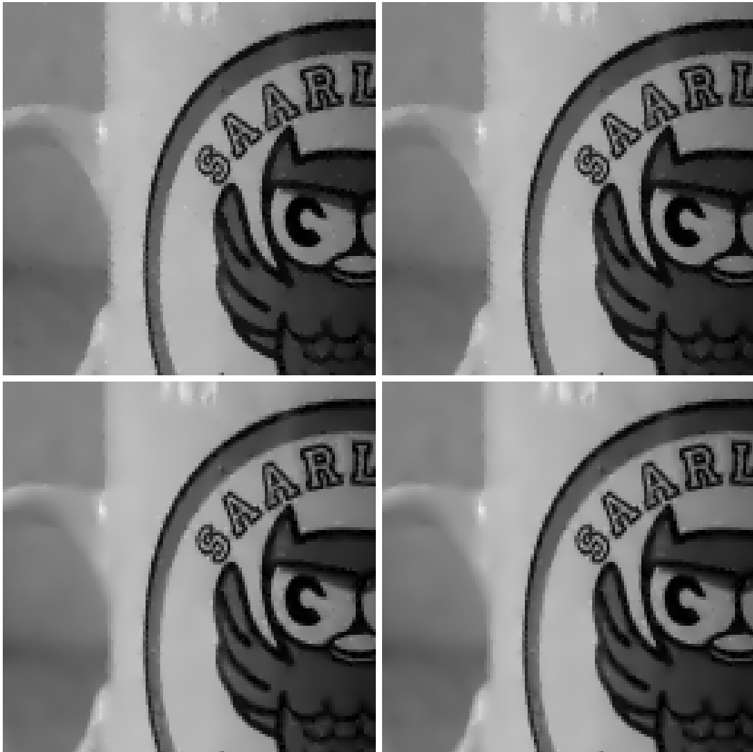
Figure 2.17: Denoising of for real-world data with Perona-Malik diffusivity g(s^2) = (1 + s^2/\lambda^2)^{-1} . Top row: Second order nonlinear diffusion. Bottom row: Fourth order nonlinear diffusion. Left column: Results with optimal \ell^1 -error. Right column: Results with optimal \ell^2 -error.
