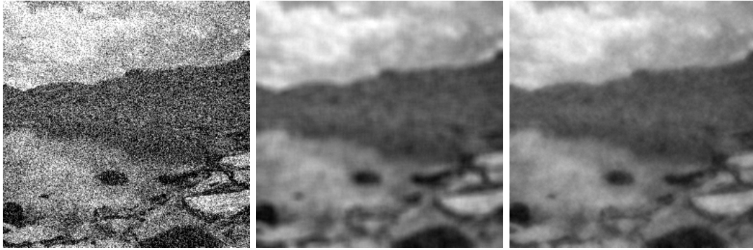
Figure 5.1: Example of the trade-off between different parameters. Left : Original image, 256 \times 256 pixels, with additive Gaussian noise with standard deviation \sigma = 50 . Middle : Denoising with E_D , radius r_D = 5 . Right : Denoising with E_C , \alpha = 0.424 .
