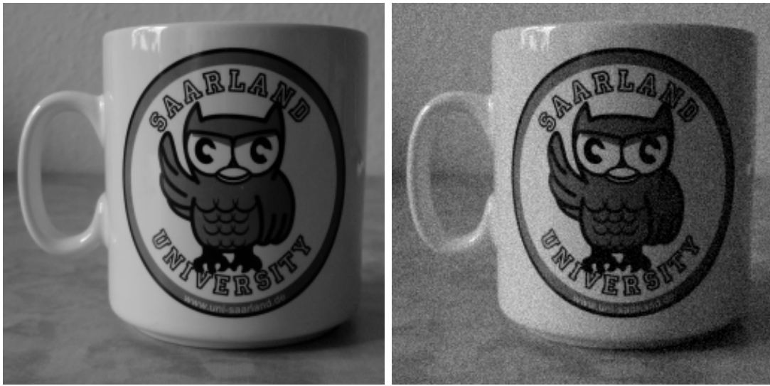
Figure 2.16: Real-world test image. Left : Original image, 256 \times 256 pixels. Right : With additive Gaussian noise, standard deviation \sigma = 10 .
