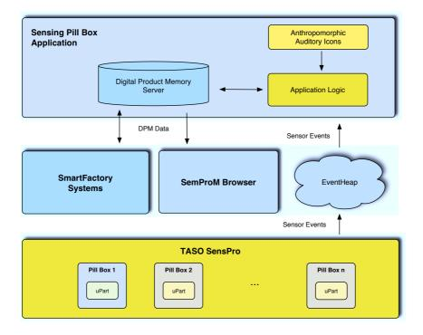
Figure 8.3: Architecture of the Sensing Pill Box based on the TASO Platform.
