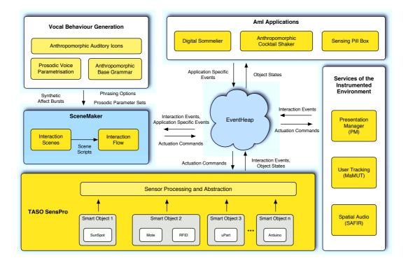
Figure 5.6: The architecture of the TASO Platform
