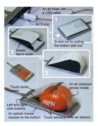
Figure 3.32: The inflatable mouse (source: [Kim et al., 2008])
