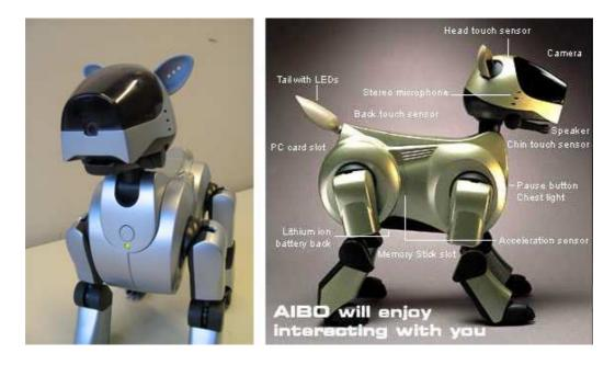
*Figure 3.42*: Sony's AIBO (sources: http://commons.wikimedia.org/ and http://www.robotstoreuk.com)
