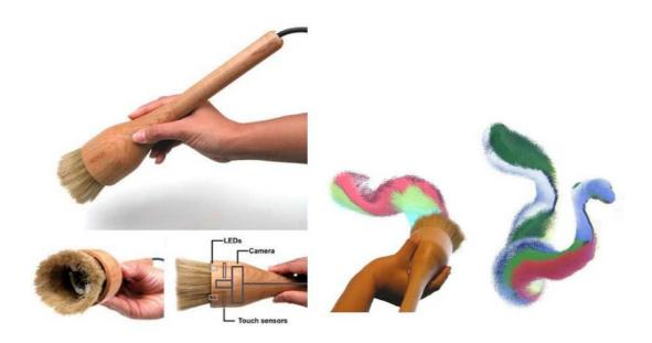
Figure 3.13: The I/O Brush (left) in action (right) (source: [Ryokai et al., 2004])
