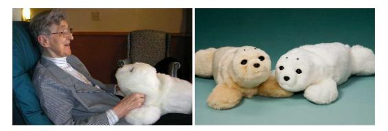
Figure 3.37: The Paro seal robot (source: http://www.parorobots.com)
