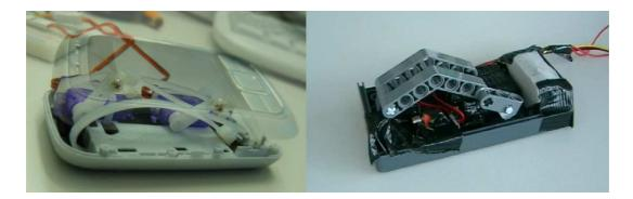
Figure 3.30: Different prototypes of the Pulsating Phone (source: [Hemmert, 2008])
