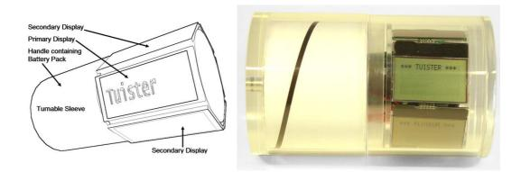
Figure 3.12: The Tuister design (left) and prototype (right) (sources: [Butz et al., 2004])
