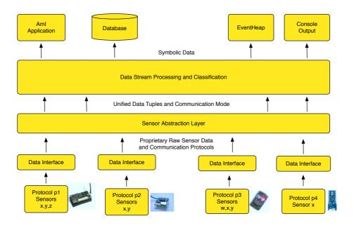
Figure 5.2: The abstraction layers of sensor stream processing in TASO SensPro
