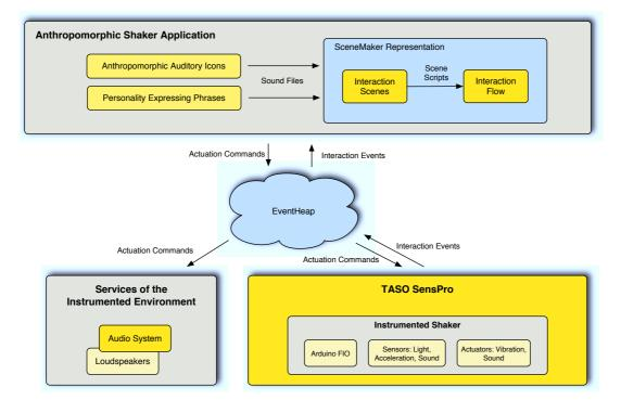
**Figure 8.13**: The overall architecture of the Anthropomorphic Cocktail Shaker based on the TASO Platform
