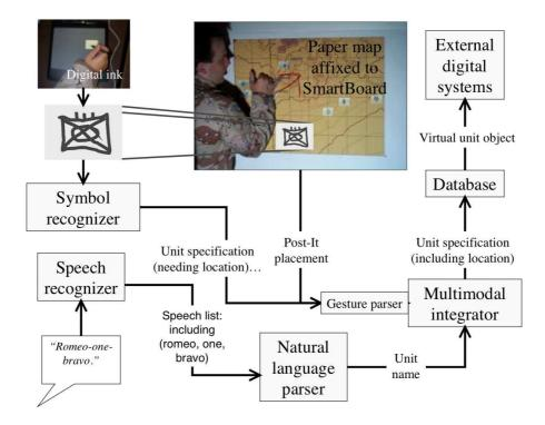
Figure 3.19: The Rasa system architecture (source: [McGee et al., 2000])
