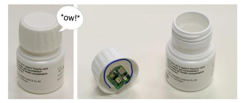
**Figure 8.1**: The Sensing Pill Box complaining when exposed to heat (left), the integrated sensor (right)
