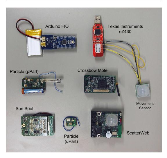
Figure 5.1: Sensor nodes experimented with during the development of TASO SensPro
