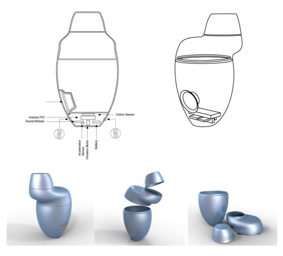
Figure 8.14: Technical drawings and 3D models of the shaker
