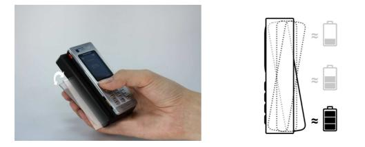
**Figure 3.35**: Left: The shape changing phone prototype - Right: A battery status indicator (source: [Hemmert et al., 2010])
