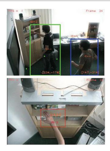
**Figure 5.8**: Macro-tracking: Person regions with position in world-coordinates, moving direction and ID (top). Micro-tracking: Skin region associated to person with ID 2 (bottom)
