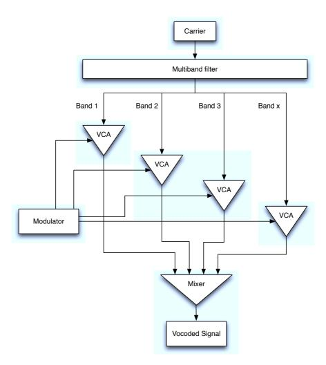
**Figure 6.2**: The vocoding principle<sup>1</sup>
