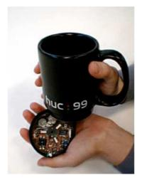
Figure 3.2: The augmented MediaCup (source: [Beigl et al., 2001])
