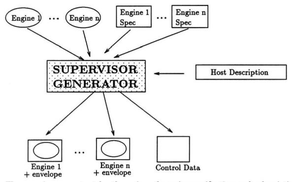
The supervisor generator takes the engines, the engine specifications and a description of the host architecture and produces the control code (engine envelope) together with the control data. The description of the host architecture contains the synchronization primitives.
