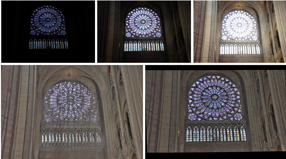
Figure 6.10: Freehand HDR imaging of a window in the cathedral Notre Dame de Paris. First row, from left to right: (a)–(c) Image 2, 4 and 6 of the exposure series (7 images, 1072 \times 712 pixels, exposure times between 1/200 and 2 seconds). Second row, from left to right: (c) Resulting tone mapped HDR image without alignment. (d) Same using our proposed alignment method.
