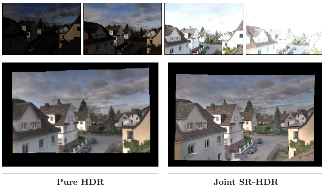
Figure 6.20: Comparing a pure HDR to a joint SR-HDR result on an outdoor scene. First row, from left to right: (a) – (d) Images 1, 4, 9 and 12 of the exposure series (12 images, 268 \times 178 pixels, exposure times between 1/2500 and 1/20 seconds.) Second row, from left to right: (d) HDR result after aligning the exposure series with our proposed technique. (e) SR-HDR result using our proposed approach. (same alignment, \vartheta = 0.2 ).
