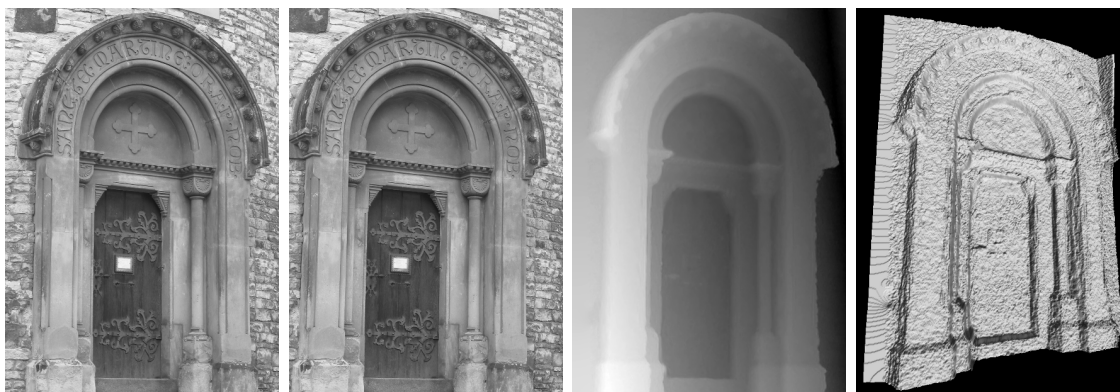
Figure 1.3: Stereo matching. From left to right: (a) Left image of the Portal scene, available at http://cmp.felk.cvut.cz/~cechj/GCS/stereo-images/Portal/ . (b) Right image. (c) Disparity estimated with our approach in [8]. (d) Corresponding reconstruction (visualising the estimated disparities as heightfield).
