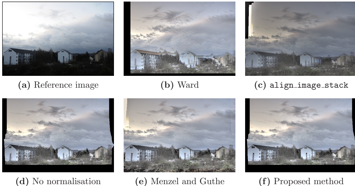
Figure 6.5: HDR imaging under severe displacements due to moving clouds and camera shake. First row, from left to right: (a) Reference image of the exposure series shown in Figure 6.4. (b) Tone mapped HDR image after alignment with the method of Ward [War03]. (c) Same using align_image_stack . Second row, from left to right: (d) Same using our method, but without data term normalisation. (e) Same using the method of Menzel and Guthe [MG07]. (f) Same using our proposed method.
