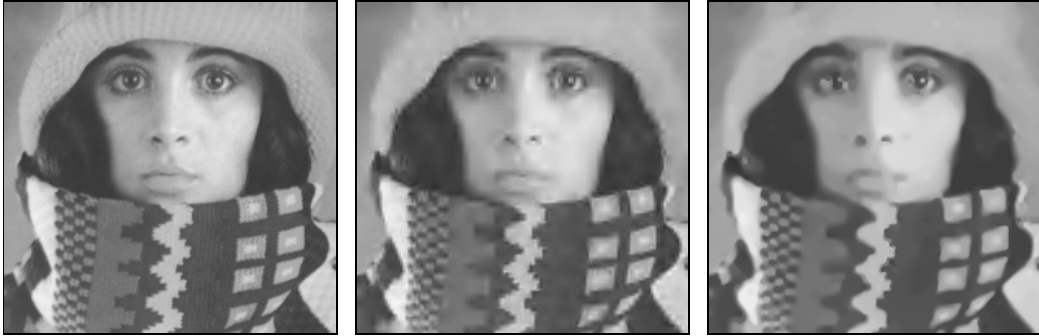
Figure 7: Left: Original image trui . Middle: Reconstructed after compression to 0.2 bpp by JPEG2000 (AAE = 4.86). Right: Reconstructed after compression to 0.2 bpp by EEDC (AAE = 4.99).
