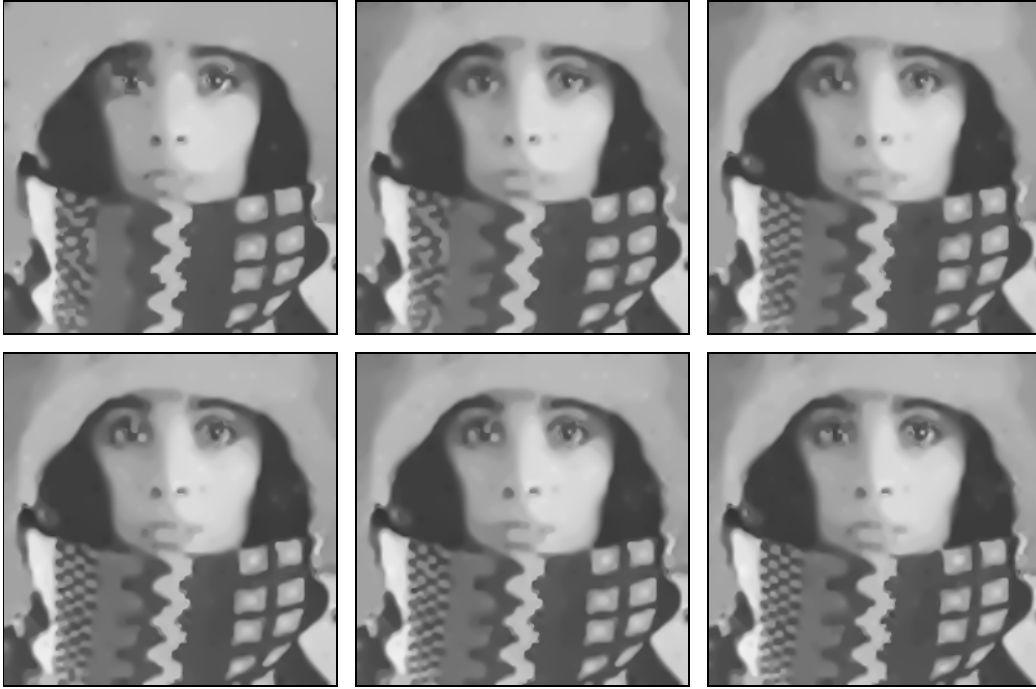
Figure 6: Comparison of BTTC-based compression methods at a compression rate of 0.2 bpp. First row, left to right: EED-based decoding (Q64+BTTC(L)-EED), with adaptive threshold (Q64+BTTC(L,AT)-EED), with EED coding (Q64+BTTC(EED,AT)-EED). Second row, left to right: with biasing (Q64+BTTC(EED,AT)+B-EED), with post-quantisation to 64 grey levels (BTTC(EED,AT)+B+Q64-EED), with post-quantisation to 32 grey levels instead (BTTC(EED,AT)+B+Q32-EED).
