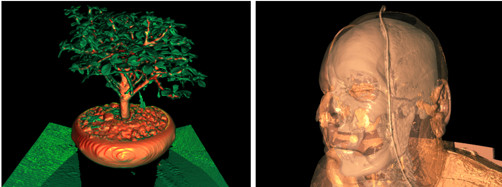
Figure 7.2: Implicitly culling non-contributing branches of the implicit kD-tree during traversal also allows for rendering multiple isosurfaces at the same time. Left: The bonsai tree, with a green isosurface for the leaves, and a brown one for the trunk. Right: The Visible Female’s head, with isosurfaces for bones and semitransparent skin.
