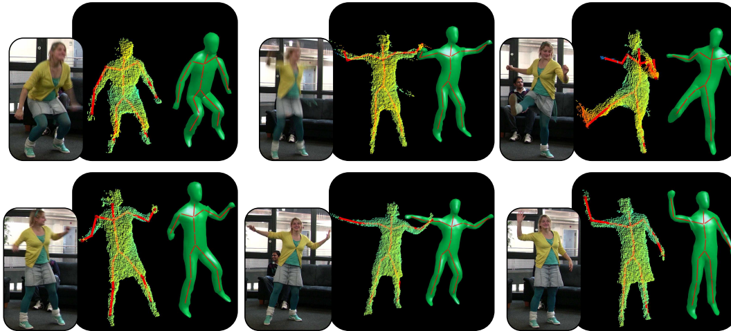
Figure 8.14. Experimental results with a different person (ToF data from a PMD camera).
