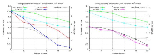
Figure 7.22. Constant stencil strong scalability Figure 7.23. Constant stencil strong scalability 44.7
