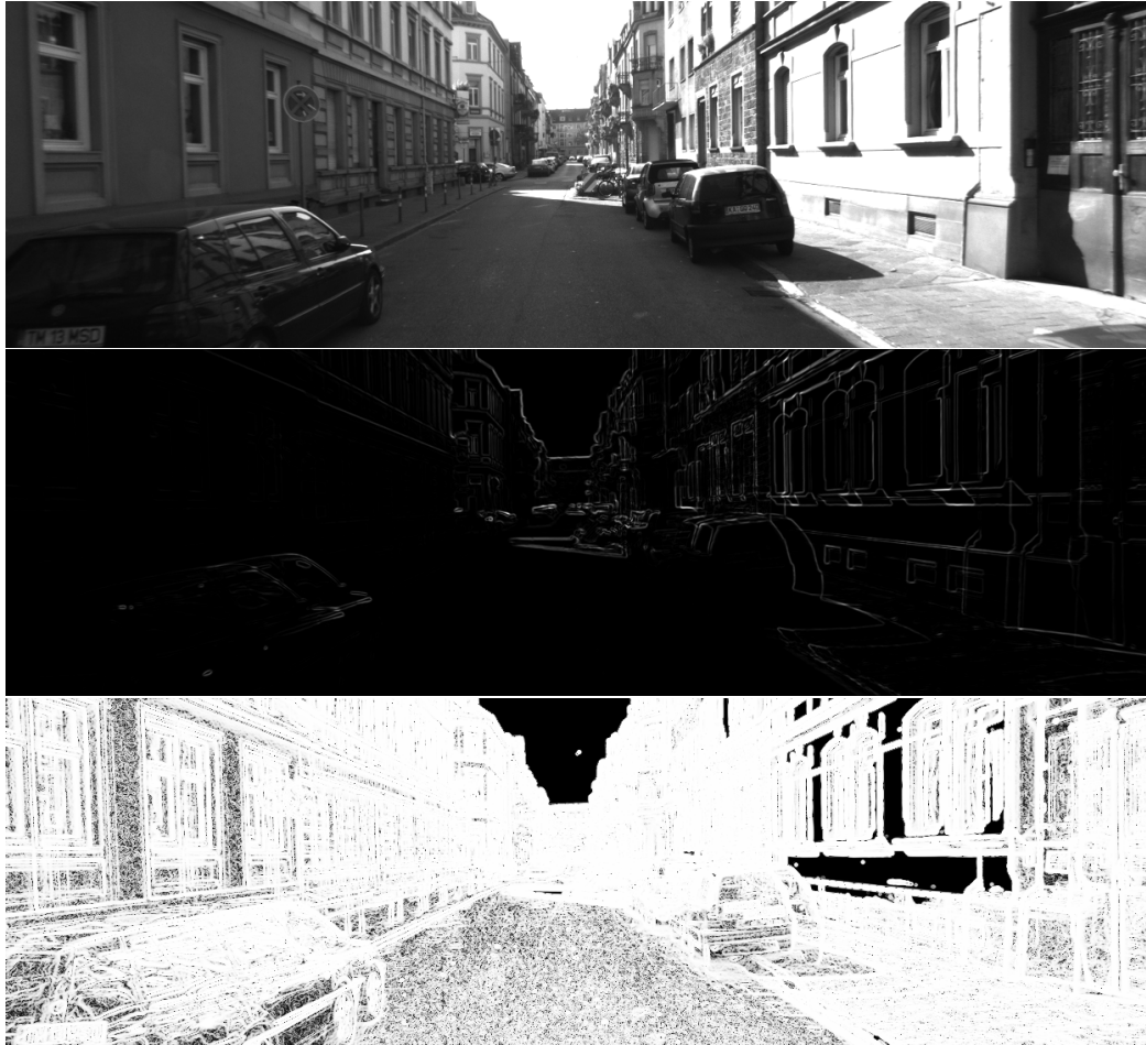
Figure 2.6: Data term normalisation. Top: First frame of KITTI training sequence #15 [Geiger et al., 2012]. Grey values are in [0, 255] . Middle: Trace of motion tensor without normalisation. Edge pixels have a clearly larger influence than pixels in smooth regions. Values are in the range [0, 25] . Bottom: Trace of motion tensor after normalisation. Values in range [0, 1] . Positions with non-vanishing image gradient all have similar weight. However, regions where the image gradient vanishes still have no influence (e.g. the sky).
