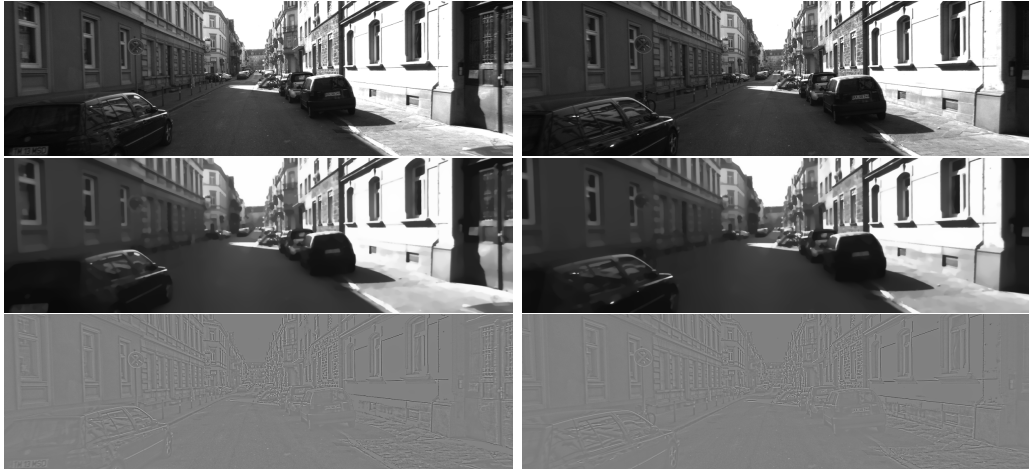
Figure 2.2: Structure-texture decomposition. Left column: Frame 1 of KITTI training sequence #15. Right column: Corresponding frame 2. Top row: Input images. Middle row: Structure part. Bottom row: Texture part.
