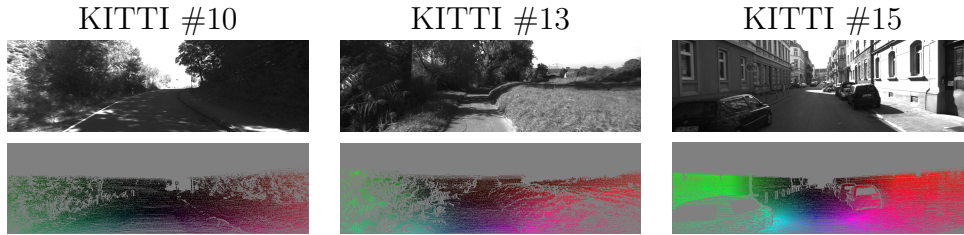
Figure 2.10: KITTI image sequences selected for the experiments of this thesis (abbreviation subset3kitti ). Unfortunately, the KITTI sequences are only available as grey value images. First frame of each image sequence with corresponding flow visualisation below it. Grey regions in the flow fields indicate occlusions or missing measurements.
