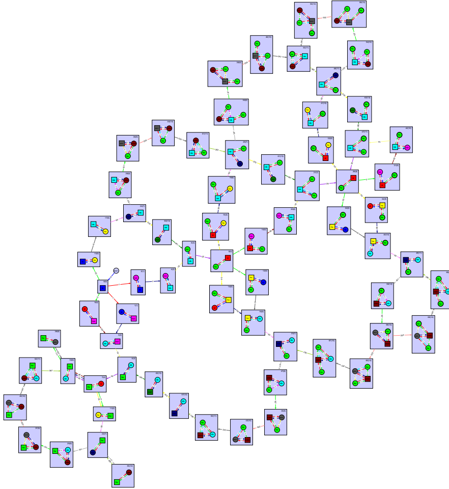
Figure 4.9: ASTRA analysis result for the synchronous merge protocol (see Section 2.3). This is a trimmed-down version showing only the most important behavior (requests are sent only when they are expected). The full version would look very chaotic. As can be seen, ASTRA already builds a labeled transition system of clusters, the theoretical foundation for which is future work. Automatic organic layout by yEd. An aesthetic appeal cannot be denied ;-)
