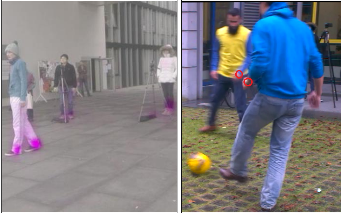
Figure 7.3: Left: Joint detection likelihoods for the right ankle in the heat-maps H_{j,c} exhibit notable positional uncertainty, and there are many false positives and close-by multiple detections. Right: Even though two body parts for the same class (i.e. lower wrist) are close to each other in the images, our approach is able to correctly estimate their individual locations.
