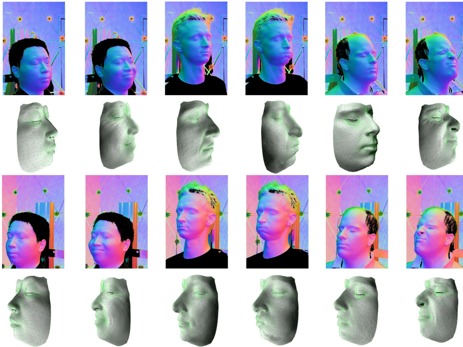
Figure 6.5: Quantitative results. Each column represents a test. For any column, the first and the third figures are two of the normal maps used in the test; The second and the fourth figures are two views of the result with normal map textured and template mesh overlapped.
