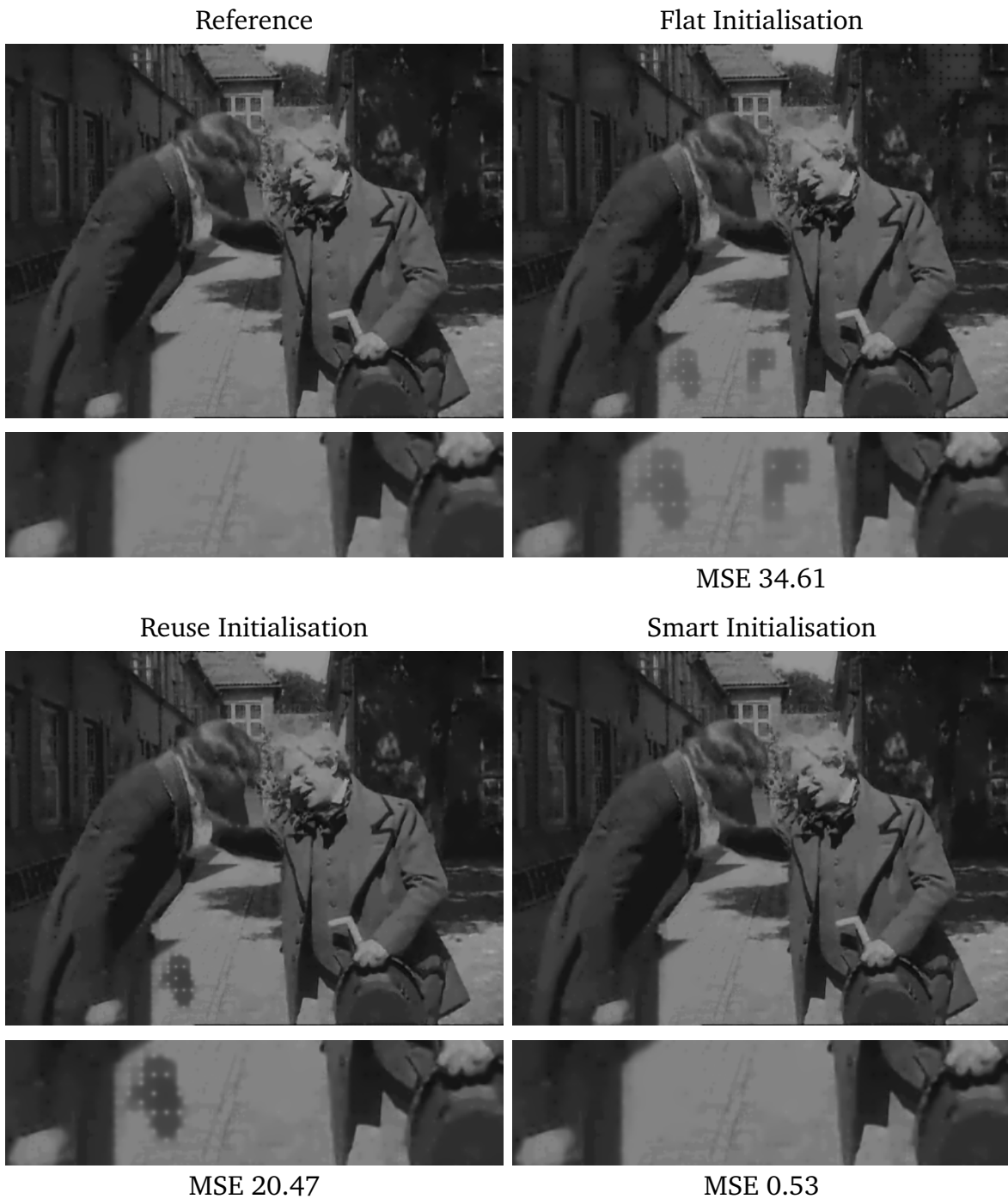
Figure 7.4.: Reconstruction of Frame 9601 based on Different Initialisations (Compression Ratio 20:1). The top row displays the reference inpainting and a reconstruction that uses a flat initialisation with the average grey value of the known pixels. In the second row, the last frame was used as initialisation on the left, and on the right linear interpolation is used in addition based on a confidence measure. Smart initialisation provides the lowest MSE for the total reconstruction.
