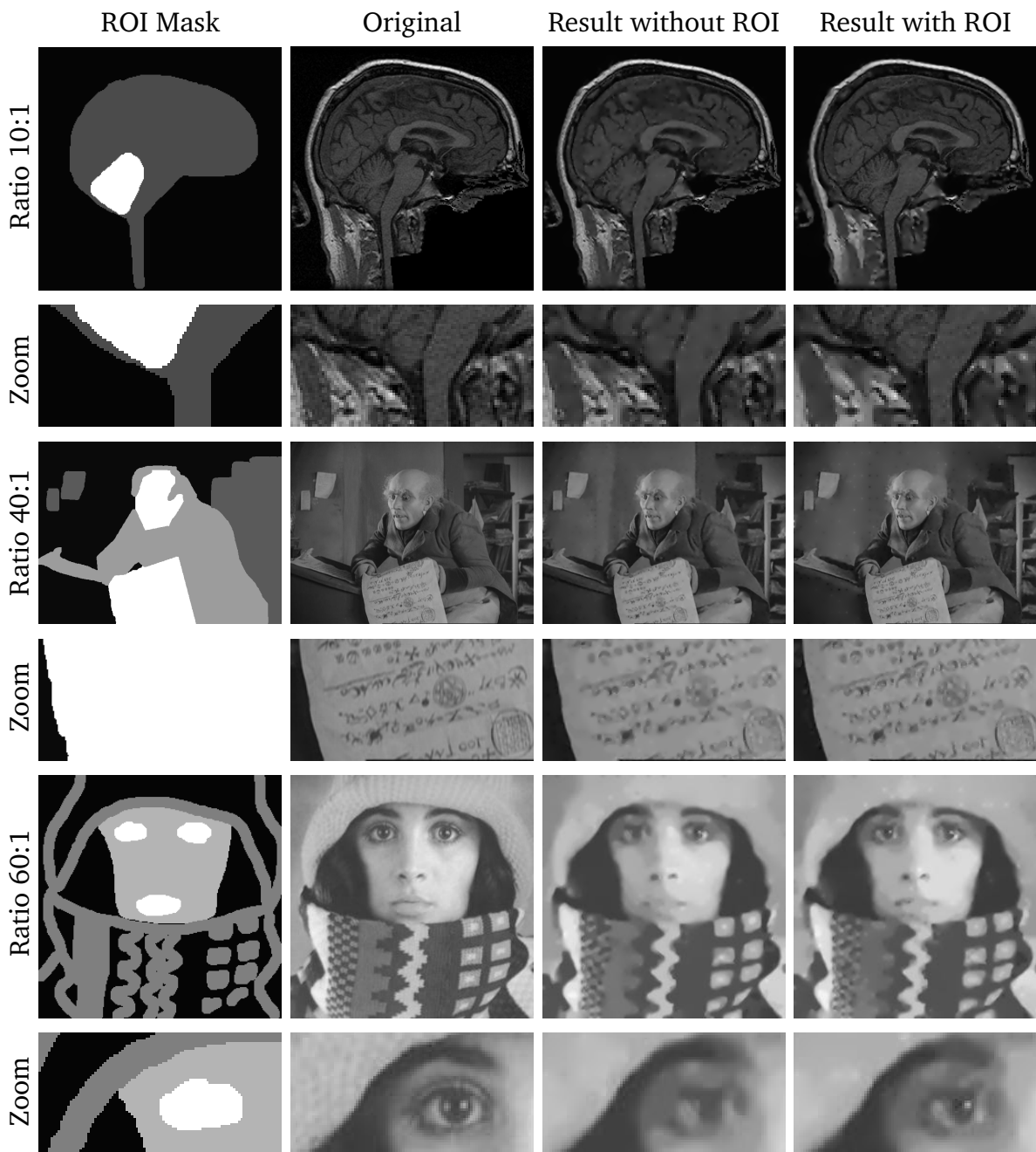
Figure 8.1.: Reconstruction Examples with and without Region of Interest Coding for the test images brain , trui , and nosferatu . The test images are ordered from top to bottom by increasing compression ratio. Bright areas in the ROI-mask have a larger weight in error computation than dark areas. For brain the ROI reconstruction is almost perfect in the cerebellum at the cost of reduced quality in other parts. Details such as text are reconstructed more accurately with ROI coding for nosferatu , while background structures are omitted. Finally, the ROI in trui allows a much higher perceived quality at high compression ratios due to better quality in facial features (in particular the eyes).
