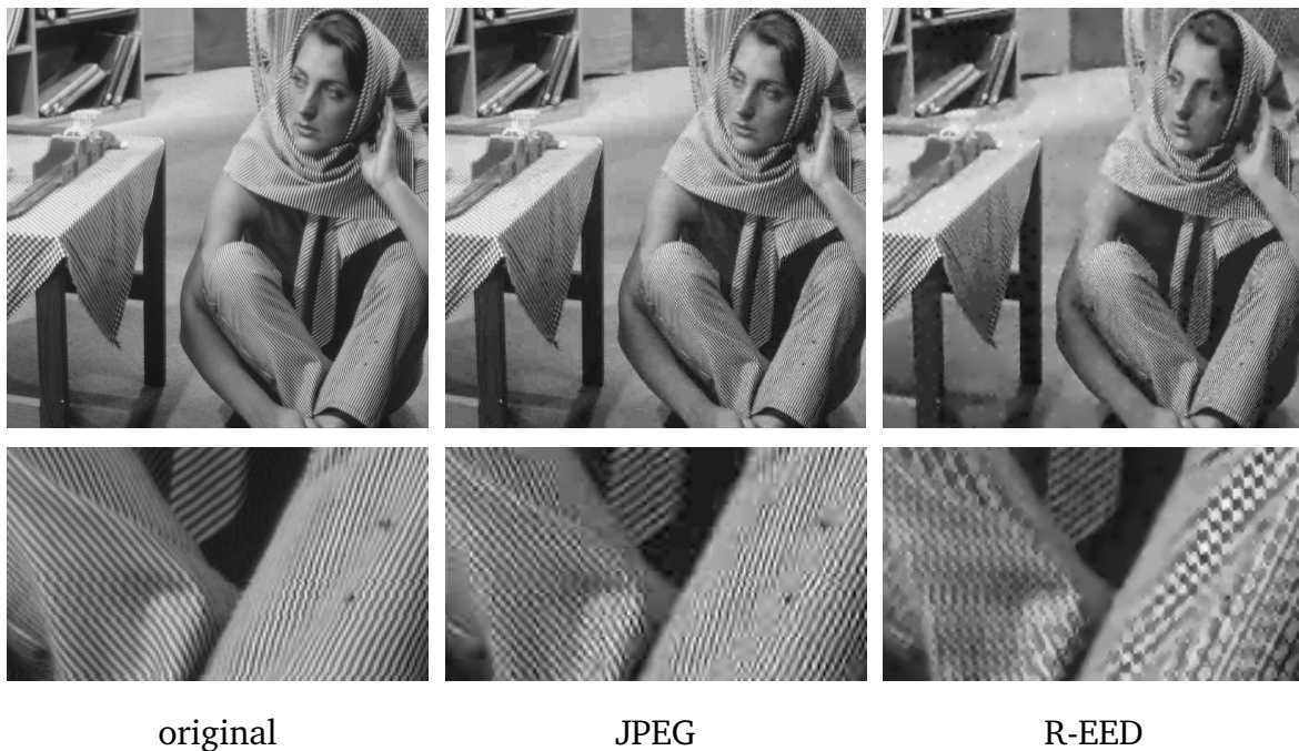
Figure 1.4.: Comparison of R-EED and JPEG on the test image barbara . As the zoom-ins in the bottom row show, R-EED does not suffer from block artefacts as JPEG does. However, JPEG still outperforms R-EED at a compression ratio of 18:1, since it can reconstruct fine scale textures.
