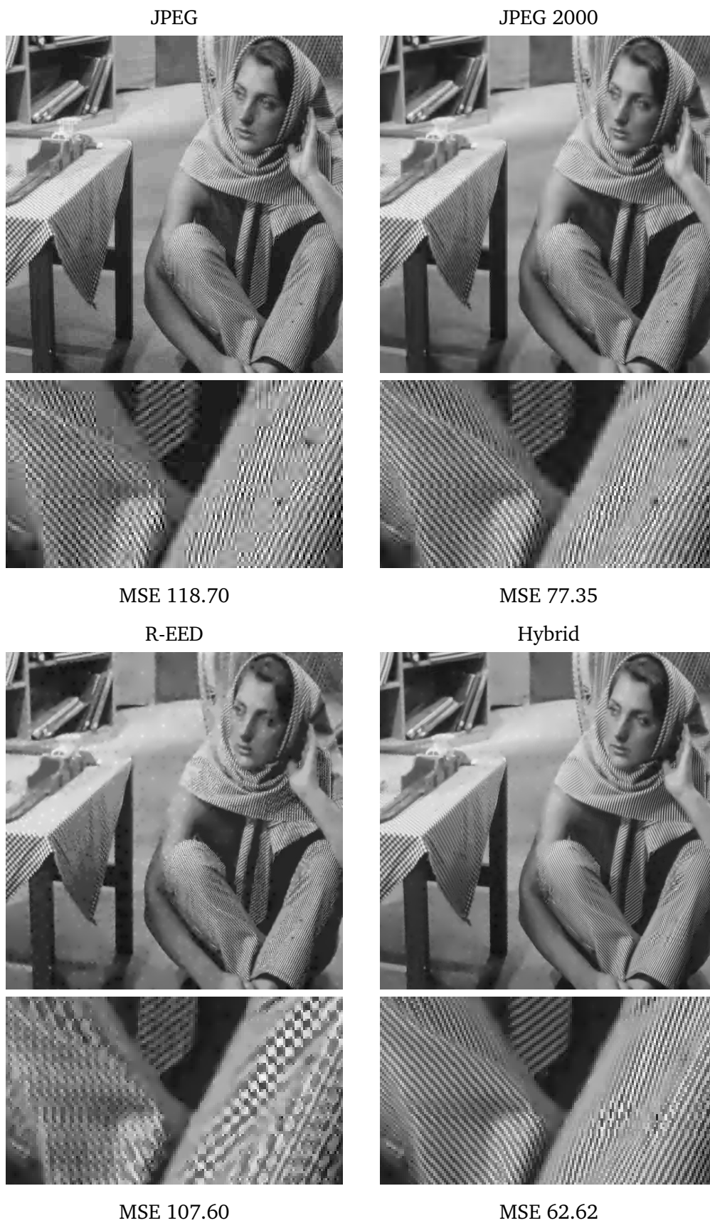
Figure 6.6.: Results for barbara with Ratio \approx 18 : 1 . The hybrid algorithm uses the upper tree limit N = 16 , block parameter b = 48 , and the NLI parameter h = 100 .
