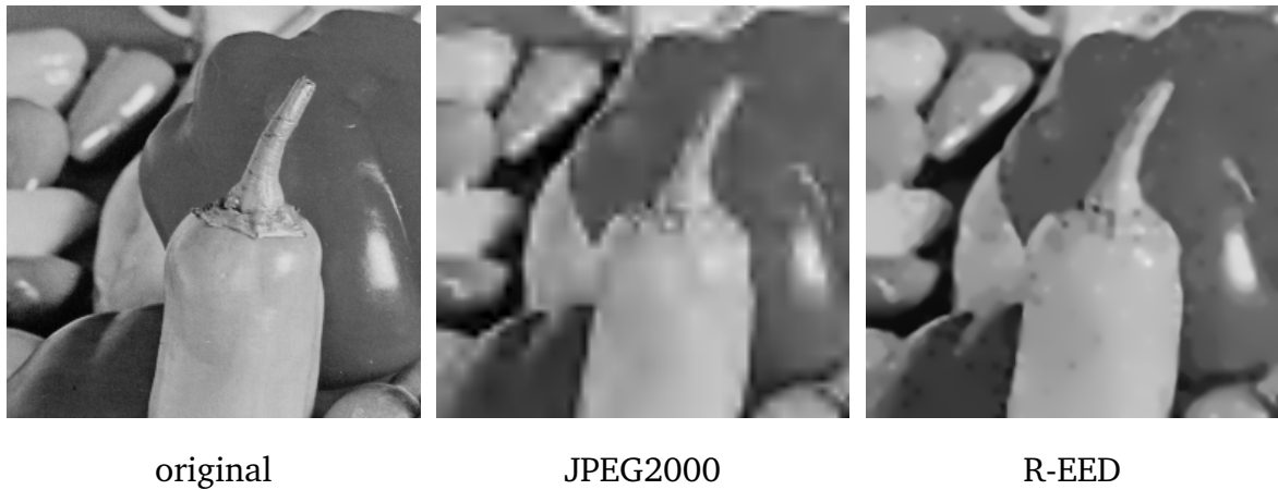
Figure 1.1.: Comparison of R-EED and JPEG2000 on the grey value image peppers . R-EED beats the quality of JPEG2000 by a considerable margin at a compression ratio of 80:1.
