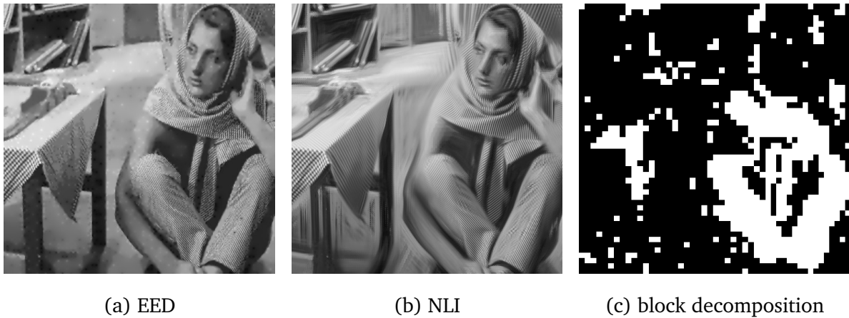
Figure 6.4.: Reconstruction of the Image barbara with EED (a) and NLI (b) from the Same Known Data. The reconstructions correspond to intermediate results from steps 1 and 2 of the hybrid algorithm for a compression ratio of \approx 18 : 1 . The block decomposition (c) with b = 48 indicates where EED (black) and NLI (white) yield better results.
