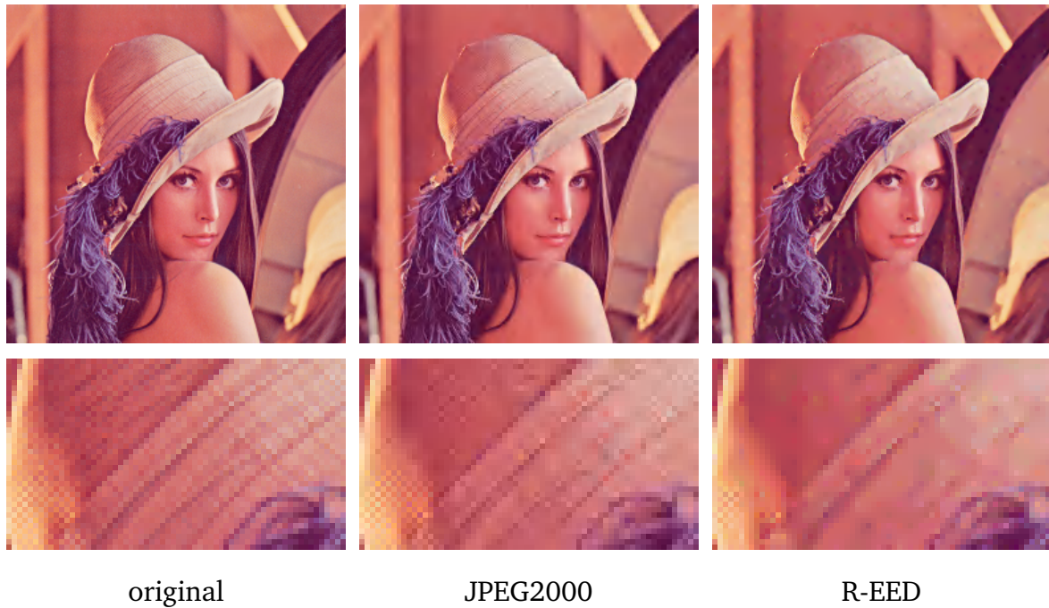
Figure 1.3.: Comparison of R-EED and JPEG2000 on the colour image lena . R-EED is not able to surpass JPEG2000 quality-wise at a compression ratio of 20:1. This is particularly obvious in the zoom-ins of the second row.
