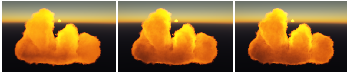
Figure 4.12: Quality comparison for different photon map resolutions, m = 100 . Left: 270 cells (0.5 MB video memory), 102k photon beams, 4.8 ms per frame. Middle: 2080 cells (4.2 MB video memory), 819k photon beams, 9.1 ms per frame. Right: 16640 cells (33.8 MB video memory), 4096k photon beams, 33.4 ms per frame. The settings used to generate the middle image are used in all the other results for the particular dataset.
