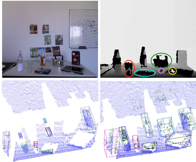
Figure 7.1: (top) Failure cases of Kinect 3D sensor: (red) transparency, (green) specularity, (cyan) dark objects under flat viewing angle, (yellow) reflections of the angle, (violet) interference of dot patterns by reflections. (bottom) We evaluate on a object segmentation task, left: result on Kinect point cloud only, right: strongly improved result on our fused estimate proposed in this chapter. (blue points: kinect; green points: cross-modal stereo)
