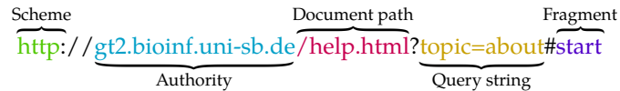
Figure 5.2: Simplified HTTP URL. Each URL consists of a scheme and scheme-specific part. For HTTP the scheme-specific part contains the host (authority), the path to the resource on the host, additional query information, and a fragment string.
