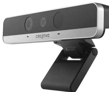
(b) The Intel RealSense camera array which adds a third spatial dimension to notebooks, tablets or smartphones
