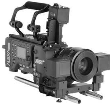
Figure 1.6: The Motion Scene Camera extending an ARRI Alexa Camera by a Depth Sensor, built by ARRI as part of the SCENE Project [24]
