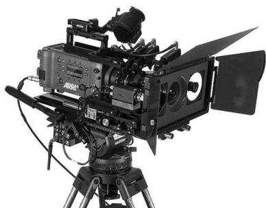
(a) A Trifocal Camera Rig combining an ARRI Alexa Camera with two Indie GS2K Cameras, build by the Fraunhofer HHI as part of the 3FLEX Project [30]
