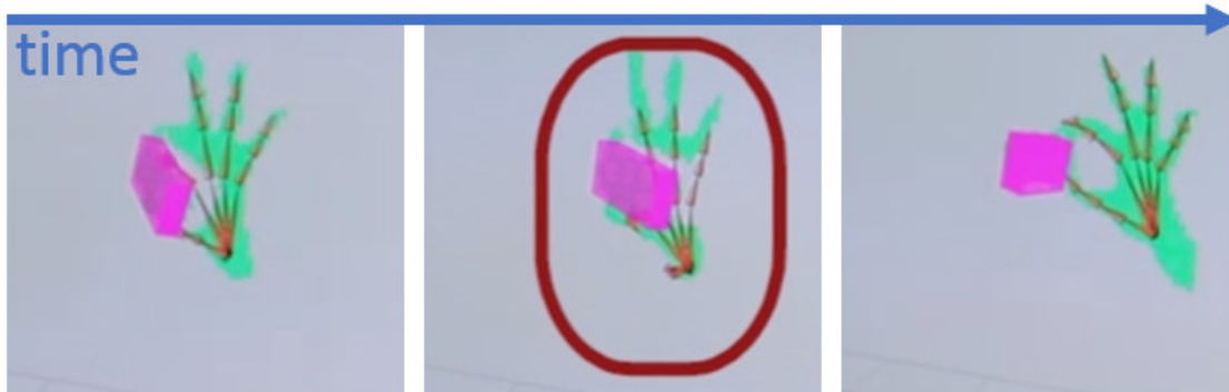
Figure 6.9 Occlusion error and recovery.
