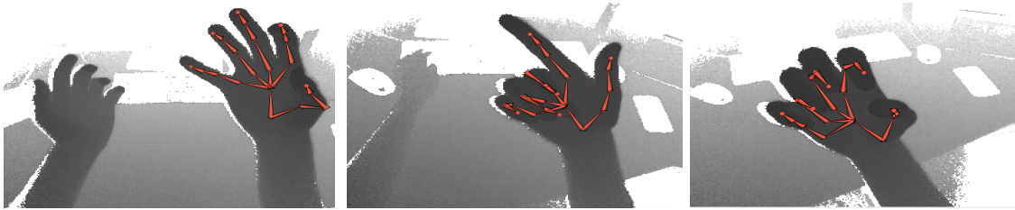
Figure 5.8 Tracking from egocentric viewpoint. Our method supports egocentric hand tracking of gestures like pointing and grasping.
