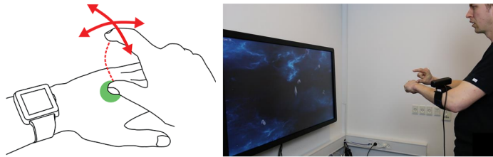
Figure 9.9 WatchSense allows for joystick-like directional control for gaming. Here a 2D spacecraft shooting game is controlled by compound Touch + Mid-air gesture. The spaceship fires when the index finger is quickly moved towards the BOH and up again.
