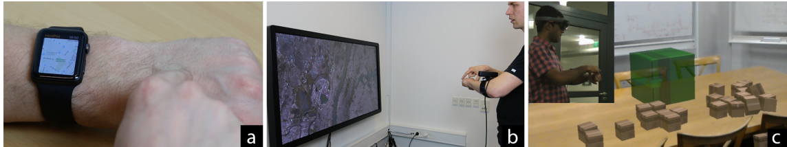
Figure 9.7 Some interactive applications enabled by WatchSense . (a) Single-touch input allows for panning a map on a smartwatch. (b) Multitouch allows for zooming/resizing a lens on a large display. (c) Compound touch and mid-air interactions allow for more expressive input for emerging mixed reality devices. Here we show a user interacting with virtual boxes through a HoloLens.
